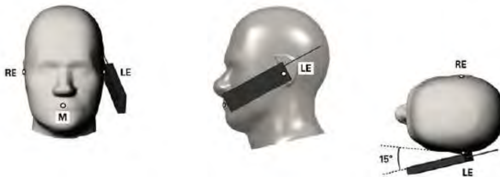
Fig.11.4 Illustration for Tilted Position
