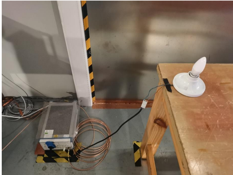
Photograph 2: Set-up for measurement of radiated emission
