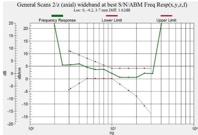
**Figure C.1 Frequency Response of CDMA BC0\_Channel 384**
