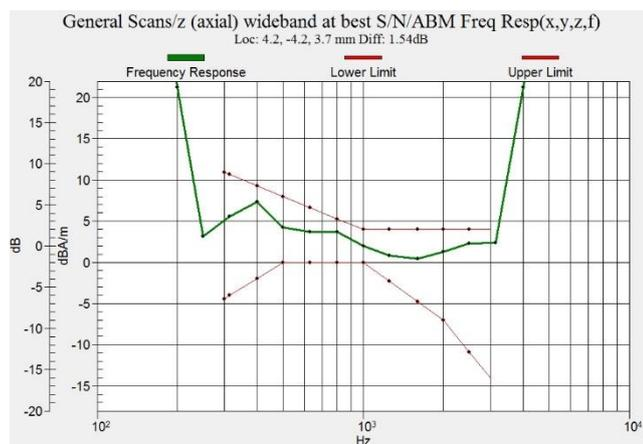
**Figure C.3 Frequency Response of CDMA BC10\_Channel 580**
