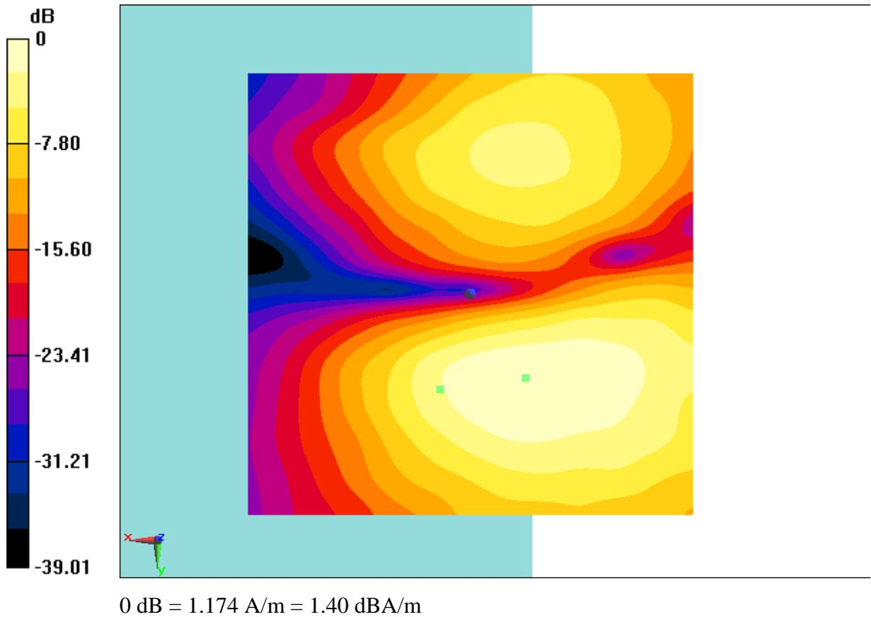
**Fig B.5 T-Coil CDMA BC10\_Channel 580**
