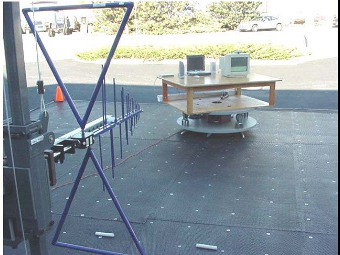
Photograph I-4 - Vertical Polarization (30MHz - 1 GHz)
