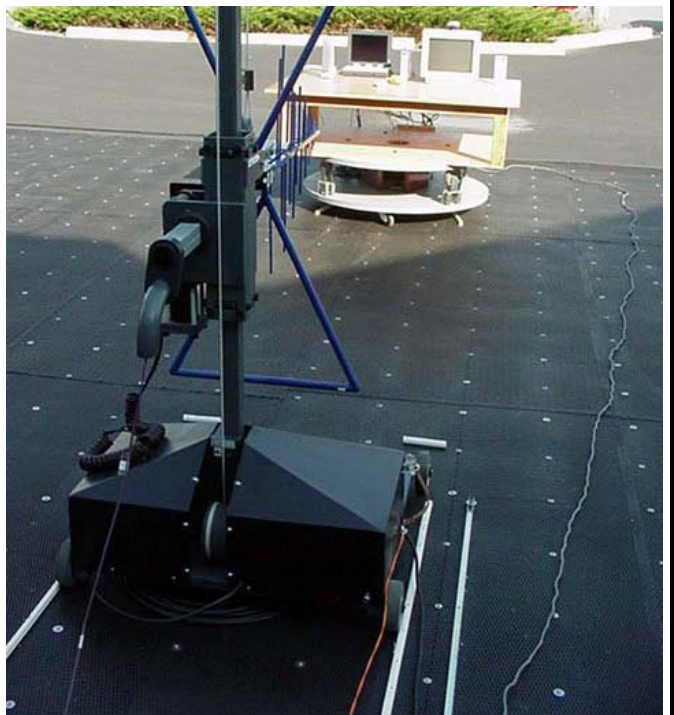
Photograph I-4 - Vertical Polarization (30MHz - 1 GHz)
