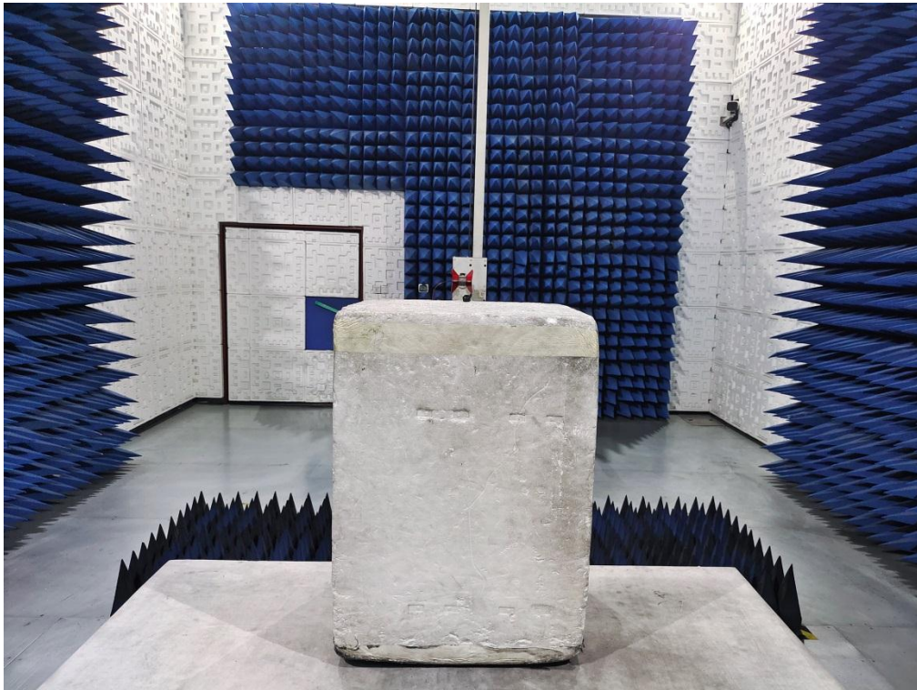
RADIATED EMISSION TEST SETUP ABOVE 1GHz
