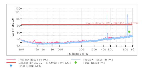
Settings: RBW = 100 kHz / VBW = 300 kHz / Sweep Time = 1s / Sweep points = 32001 The peak on the left above the limit is the SRD 400 MHz (450.5 MHz) carrier frequency. The peak on the right above the limit is the 3G V (846.6 MHz) carrier frequency.
