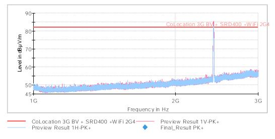
Settings: RBW = 1 MHz / VBW = 3 MHz / Sweep Time = 1s / Sweep points = 32000 The peak above the limit is the WLAN 2.4 GHz (2412 MHz) carrier frequency.
