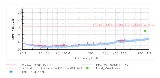
Settings: RBW = 100 kHz / VBW = 300 kHz / Sweep Time = 1s / Sweep points = 32001 The peak above the limit is the SRD 400 MHz (450.5 MHz) carrier frequency.
