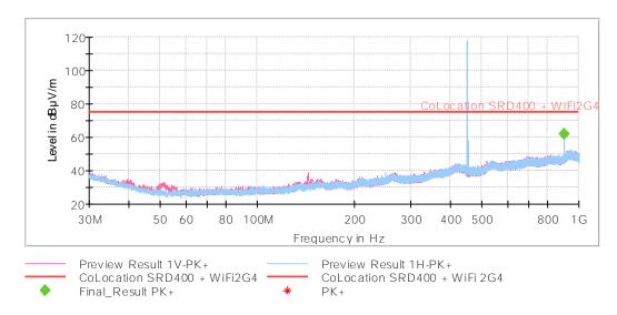
Settings: RBW = 100 kHz / VBW = 300 kHz / Sweep Time = 1s / Sweep points = 32001 The peak above the limit is the SRD 400 MHz (450.5 MHz) carrier frequency.
