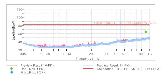
Settings: RBW = 100 kHz / VBW = 300 kHz / Sweep Time = 1s / Sweep points = 32001 The peak above the limit is the SRD 400 MHz (450.5 MHz) carrier frequency.
