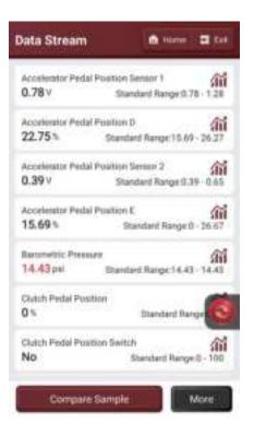
When the data stream options are not displayed in the screen, scroll up and down to view all the options. There are three display modes, you can choose the most suitable way to browse:
