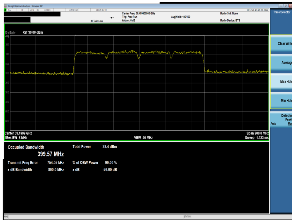
Plot 7-414. Ant M0 OBW (Band n260-100MHz-4CC MIMO CP-OFDM – QPSK – Mid Channel)
