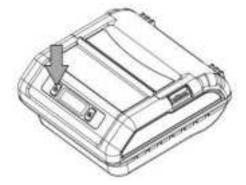
Press and hold both the MODE & FEED. Release the buttons after printer displays "Language: English", you can configure the settings.
