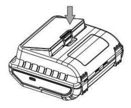
3. To remove the battery back, pull back the hook, and use the opposite procedure from the one you used to insert the battery pack.
