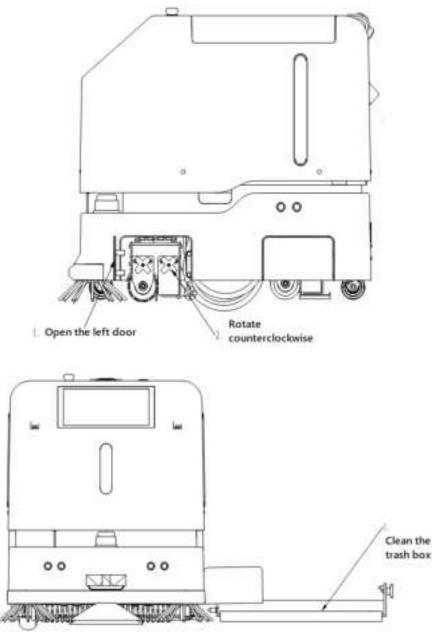
2. Filter tank and sewage box cleaning
