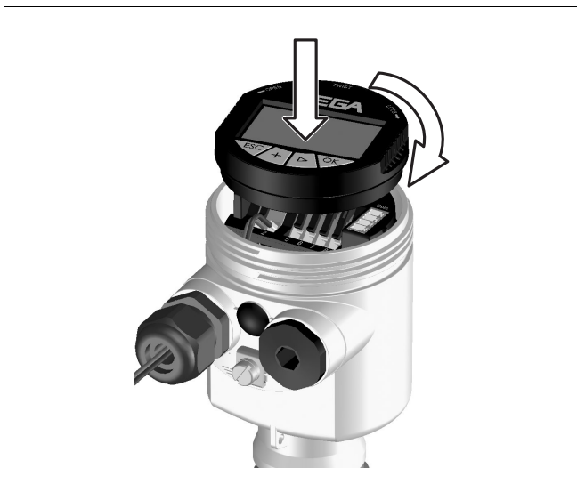
Fig. 26: Installation of PLICSCOM
