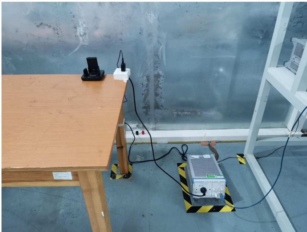
Conducted Emission-AC adapter charge mode
