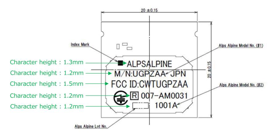
The above characters are engraved on the cover of the module. Therefore, it cannot be easily peeled off.
