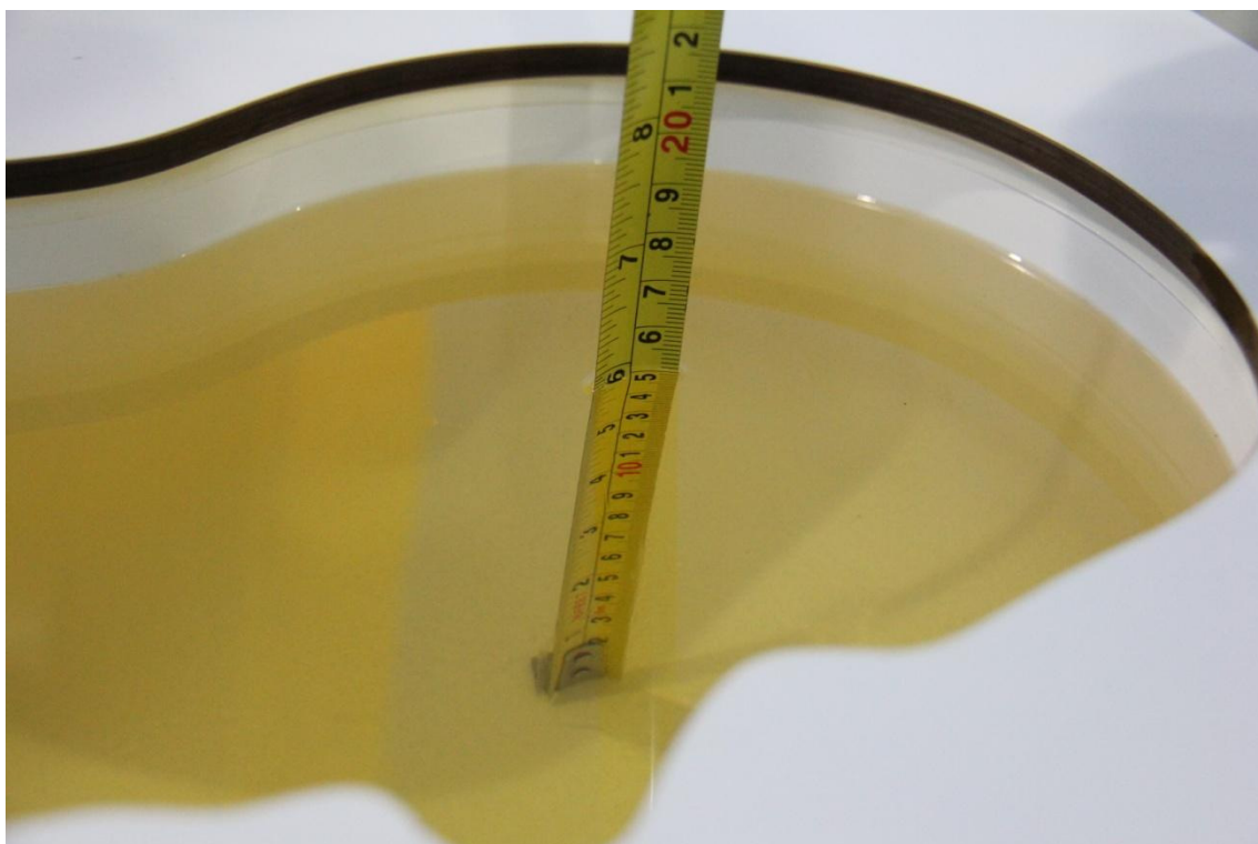
Picture 7-3: Liquid depth in the Head Phantom (835 MHz)
