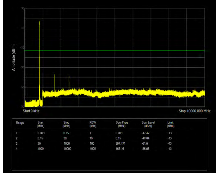
Band5 16QAM BW=3MHz Channel=20525 RB Size=15 Position=#0
