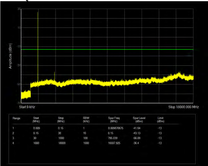
Band4 16QAM BW=1.4MHz Channel=20393 RB Size=6 Position=#0
