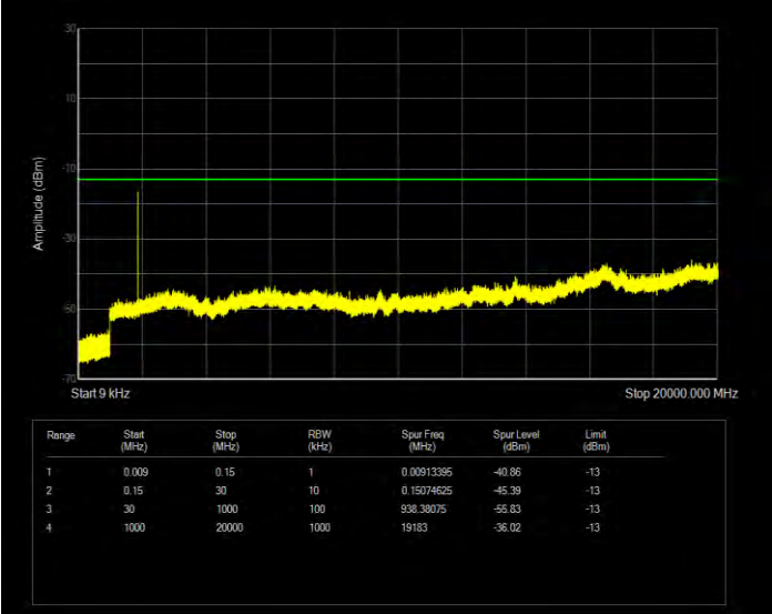
Band2 16QAM BW=1.4MHz Channel=19193 RB Size=6 Position=#0
