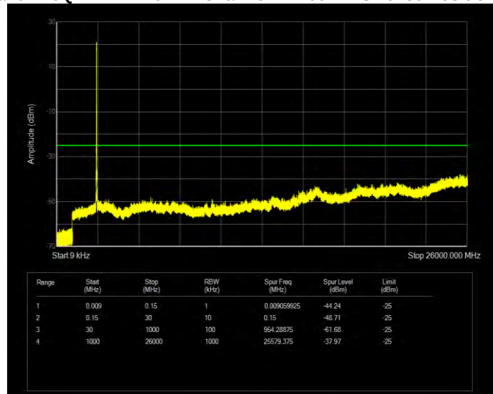
Band7 16QAM BW=10MHz Channel=21400 RB Size=50 Position=#0
