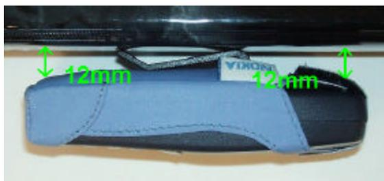
Picture 2. Separation distance with Carry Sleeve CSH-7
