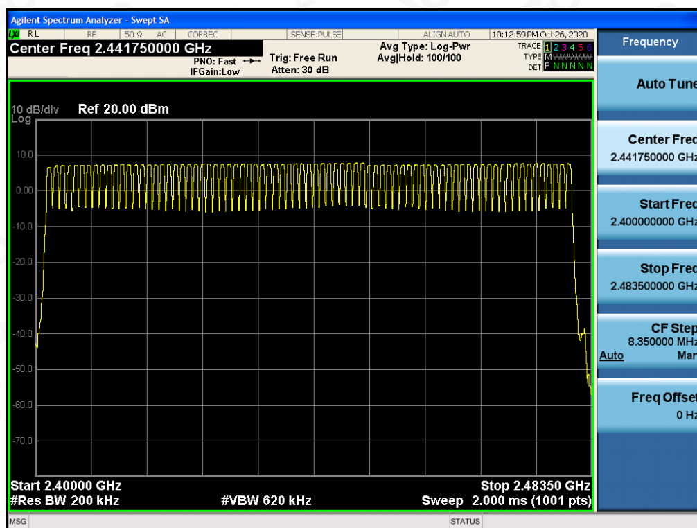
TEST PLOT FOR NO. OF TOTAL CHANNELS
