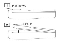
Press the battery release button located in the back of the battery pack.
