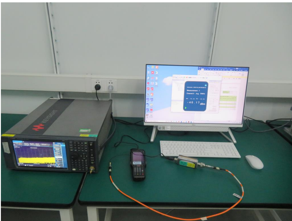
Description: RF Conducted Test Setup
