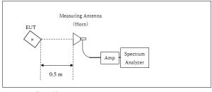
Distance Factor:  $20 \times \log (0.5 \text{ m}^* / 3.0 \text{ m}) = -15.6 \text{ dB}$ \*Test Distance: 0.5 m
