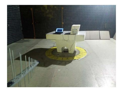
$\label{eq:Photograph No.4} Photograph No.4 \\ Spurious emissions measurement setup in the anechoic chamber in 1 – 18 GHz$
