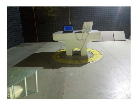
$\label{eq:Photograph No.5} Photograph No.5 \\ Spurious emissions measurement setup in the anechoic chamber in 18 – 27 GHz$
