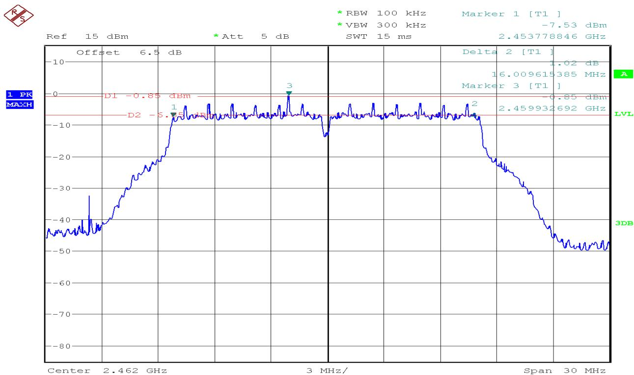
IEEE 802.11n HT20 mode / Chain 06dB Bandwidth (CH Low)
