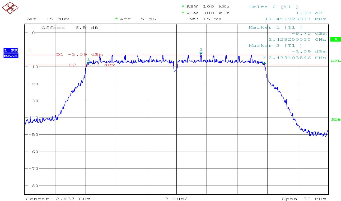
**6dB Bandwidth (CH High)**
