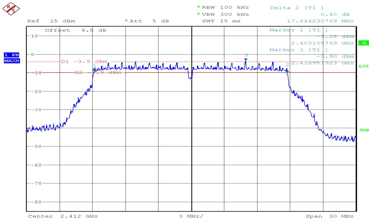
**6dB Bandwidth (CH Mid)**
