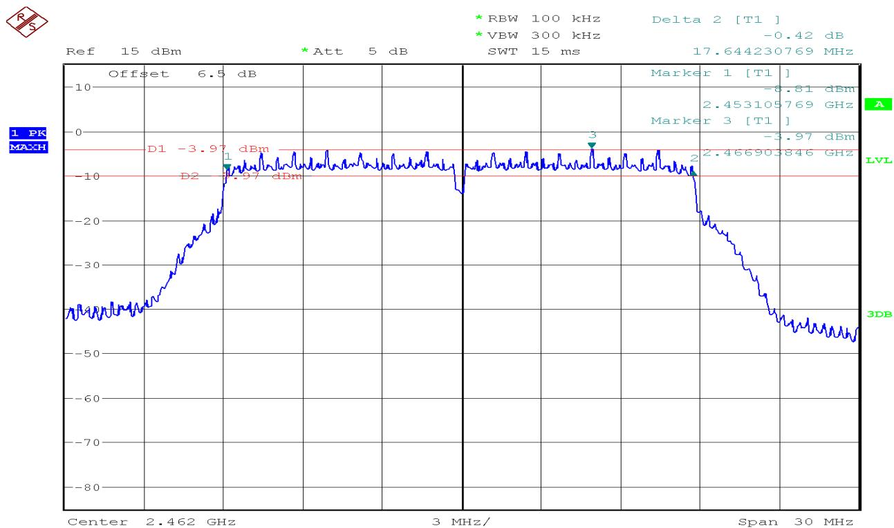
**IEEE 802.11n HT40 mode / Chain 0****6dB Bandwidth (CH Low)**
