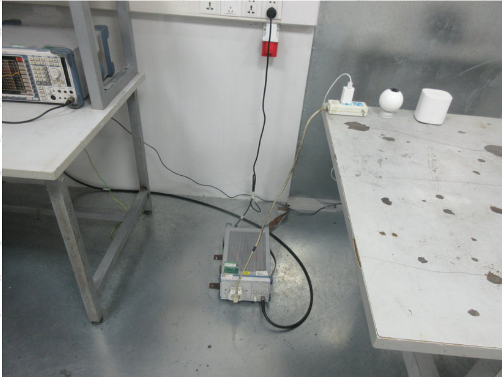
Photo of Power Line Conducted Emission Test
