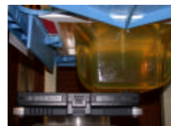
Figure B.2 Body SAR Test Setup -- Lap Position --
