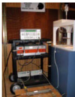
Figure A.0 Dipole Validation Test Setup
