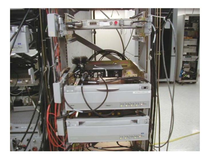
Radio setup for the Spurious Emission at Antenna Terminals
