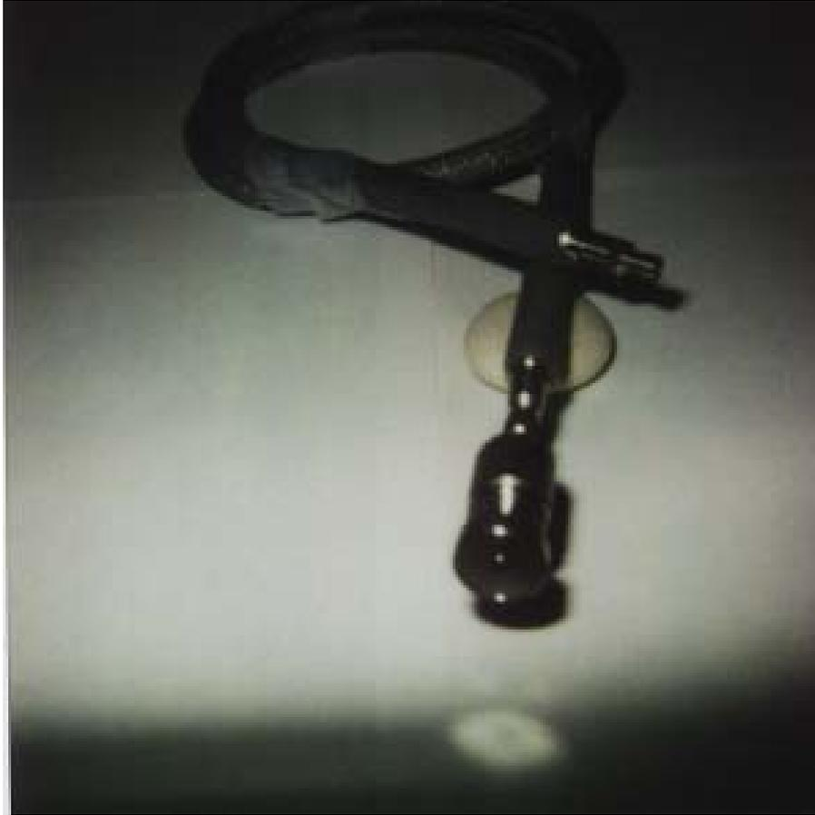
Fig. 17. Photograph of the Hewlett Packard Model 85070B Dielectric Probe. This is an open-circuited coaxial line probe.
