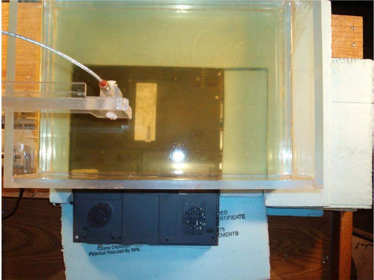
Fig. 4. Photograph of the bottom of Quantatw Model ZG1S PC pressed against the base of the planar phantom. This is **Configuration 1** for SAR testing. This Configuration 1 was also used for Quantatw Model Z11S and Compal Model L1S PCs with the bottom of each of the PCs pressed against the base of the planar phantom.
