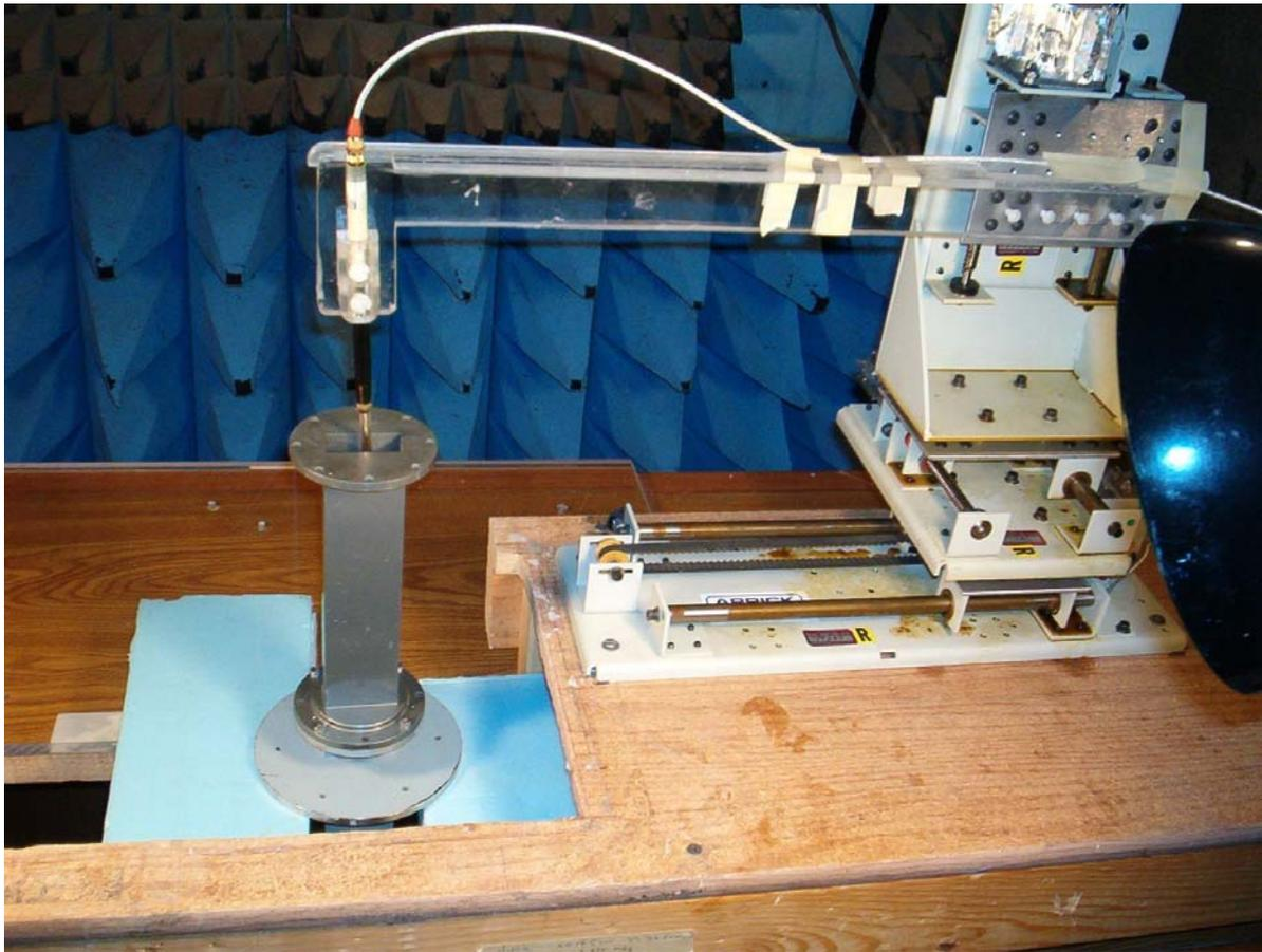
Fig. 13a. A photograph of the waveguide setup used for calibration of the Narda Model 8021 E-field probe in the frequency band 5.2-5.8 GHz.
