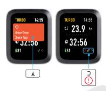
MasterMind H3 has a built-in diagnostic system to automatically check and identify the functionality of the system. If the system detects an error, it shows on the display. In some cases, the error message can be dismissed by pushing any button on the remote. When dismissed, the icon appears in the lower notification bar.
