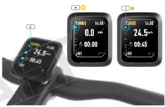
The Garmin radar system is integrated into the MasterMind H3 display and appears on the left side of the display on equipped models (A).
