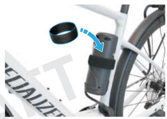
Insert the RE into the bottle cage, then secure the RE into the bottle cage, using the supplied Specialized battery retention band.
