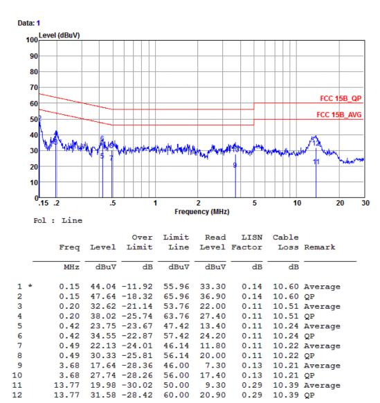
Remarks: 1. Measured = Reading + Lisn Factor + Cable Loss.
