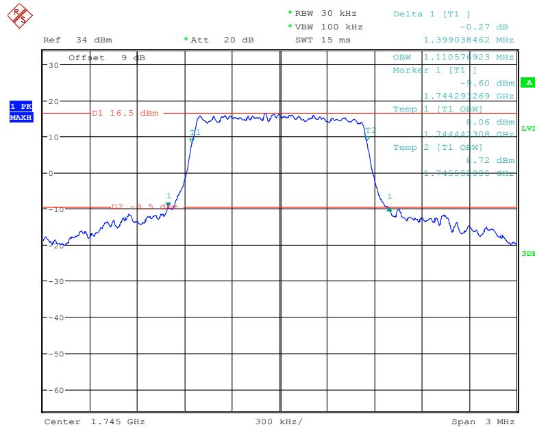
**16-QAM (1.4 MHz) - 26 dB Bandwidth & 99% Occupied Bandwidth, Middle channel**
