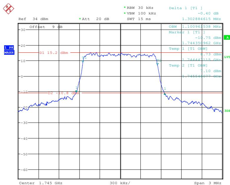
**QPSK (3.0 MHz) - 26 dB Bandwidth & 99% Occupied Bandwidth, Middle channel**
