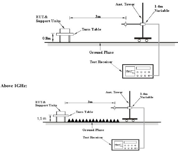
The radiated emissions were performed in the 3 meters distance, using the setup accordance with the ANSI C63.10-2013. The specification used was the FCC 15.205, 15.209, and FCC 15.231 limits.
