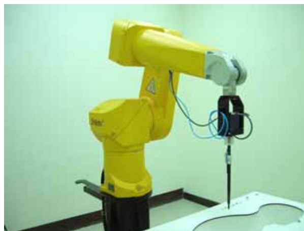
Fig. 5.2 Probe setup on robot
