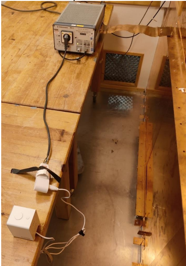
Test setup for conducted emission 150 kHz – 30 MHz
