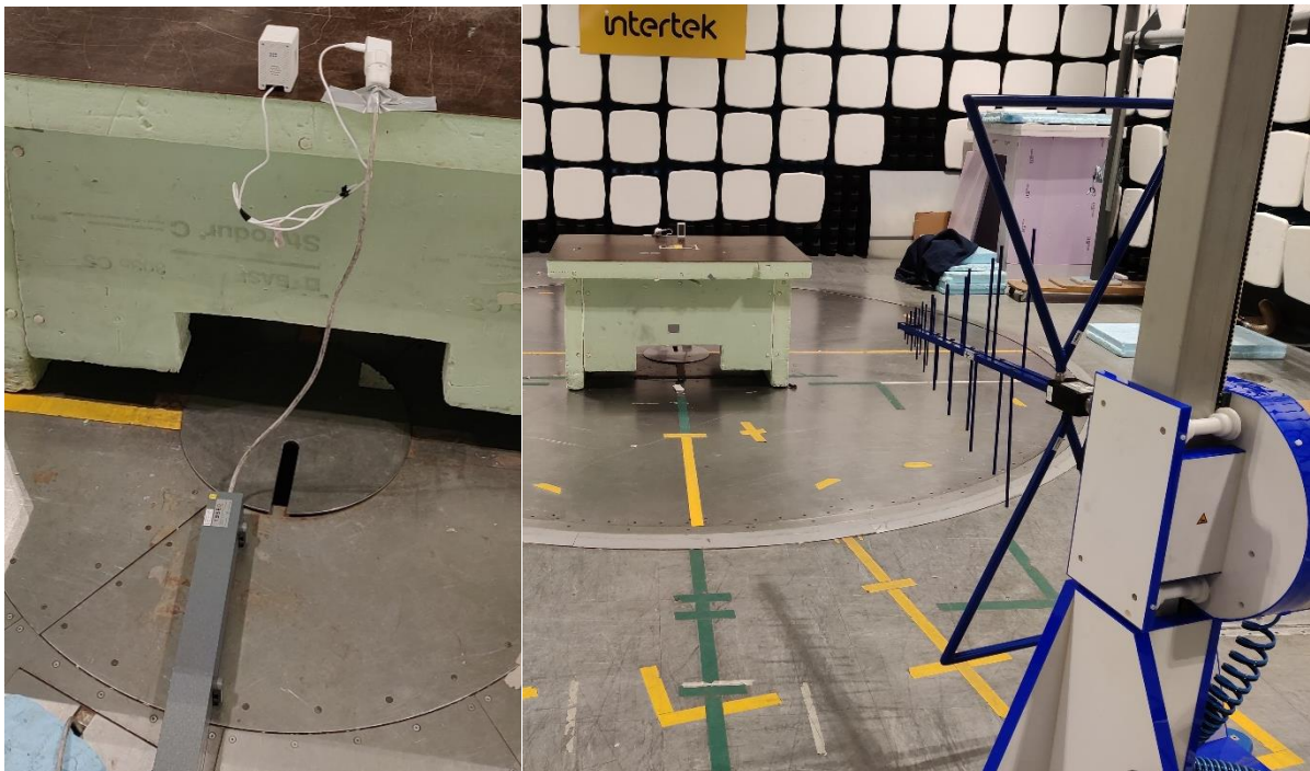
Test set up radiated emission 30 MHz – 1 GHz
