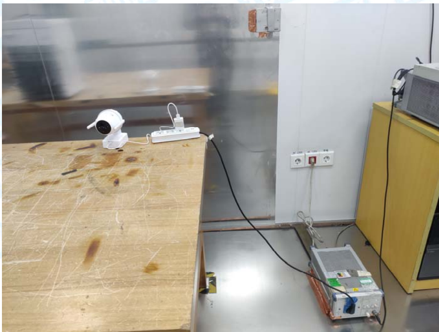
Photo of Setup for Conducted Emission
