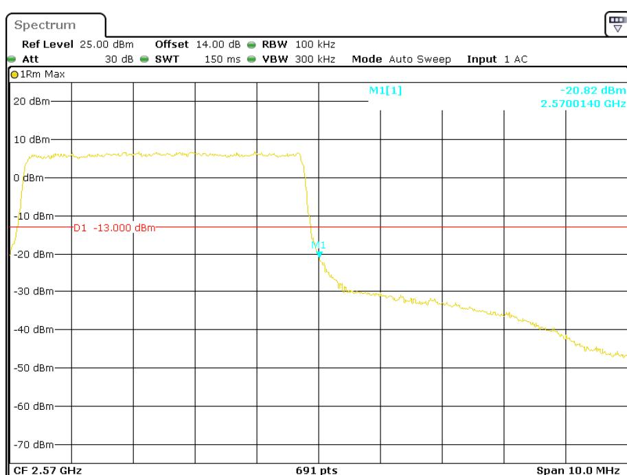
**QPSK (10.0 MHz, FULL RB) - Left Band Edge**
