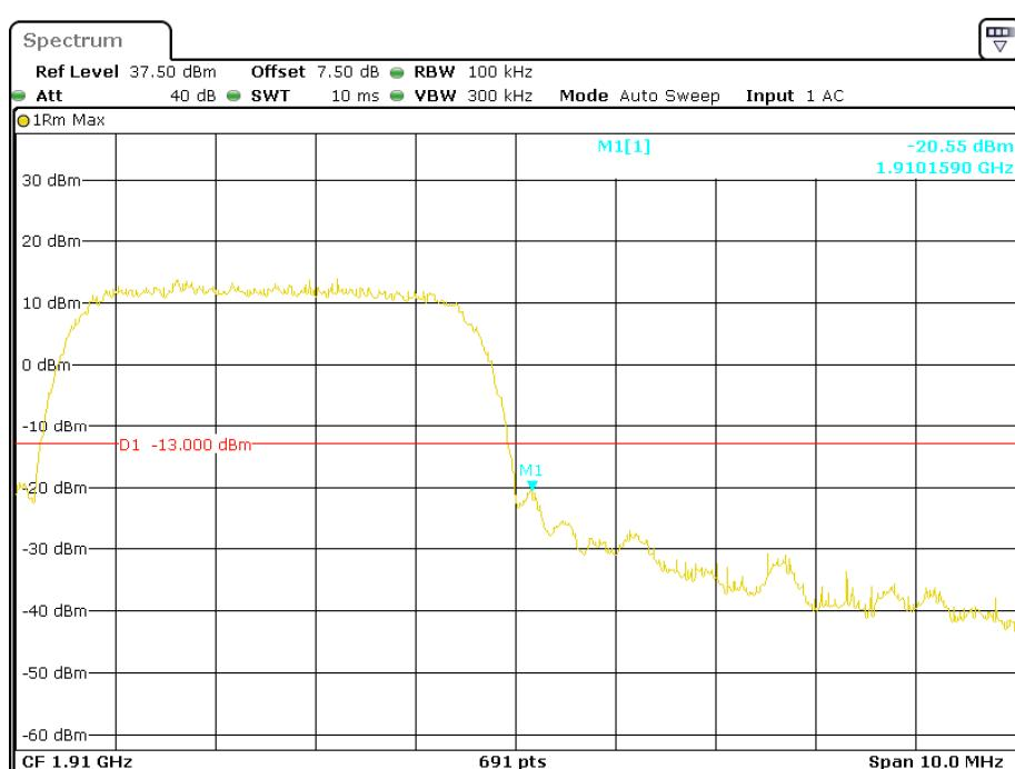
**PCS Band, Left Band Edge for HSDPA (16QAM) Mode**
