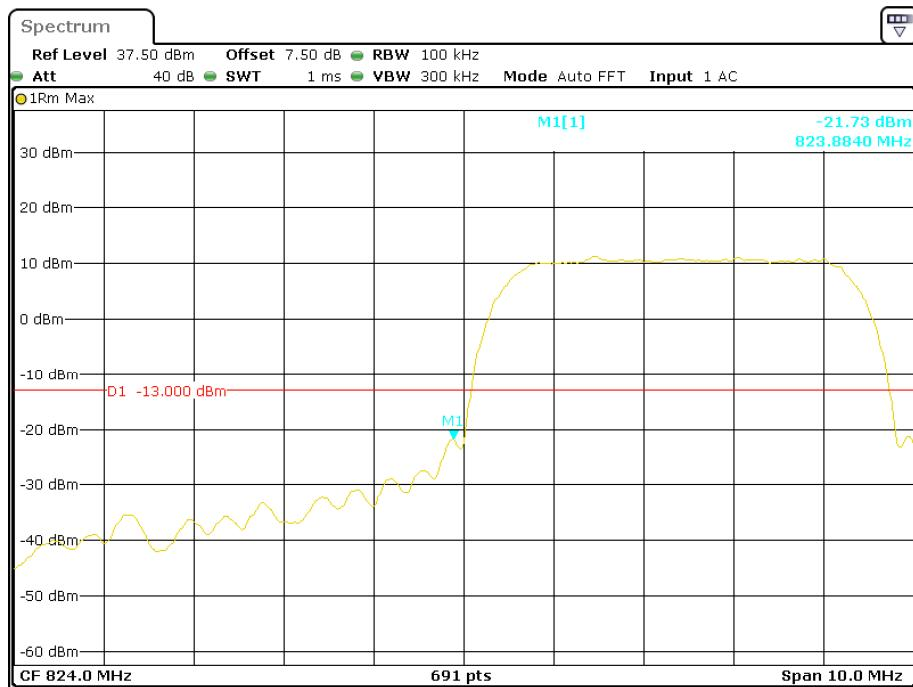
**Cellular Band, Right Band Edge for HSDPA (16QAM) Mode**
