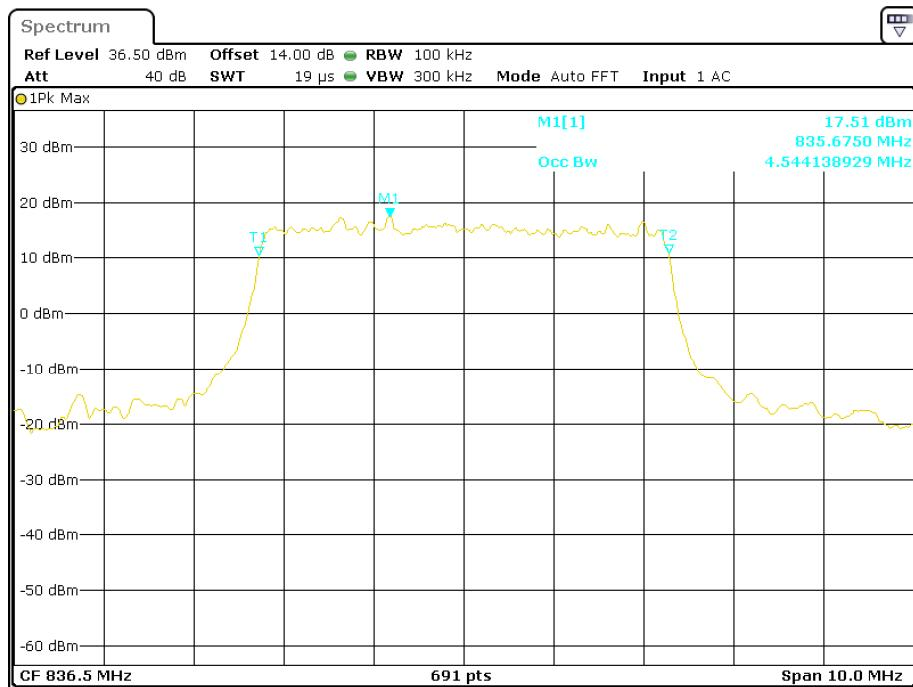
**16-QAM (5.0 MHz) - 99% Occupied Bandwidth, Middle channel**
