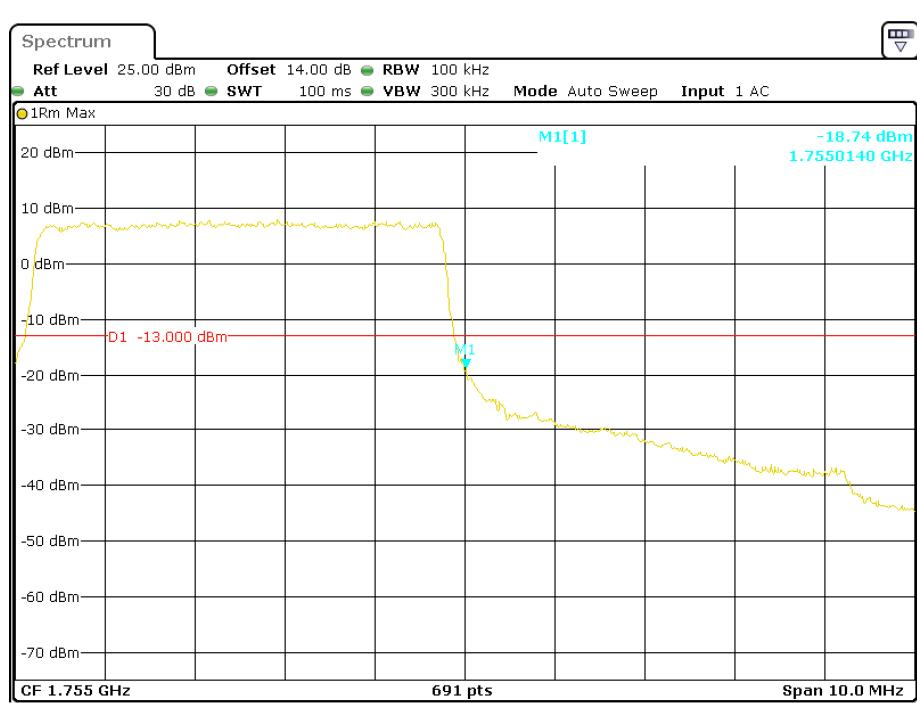
**QPSK (10.0 MHz, FULL RB) - Left Band Edge**
