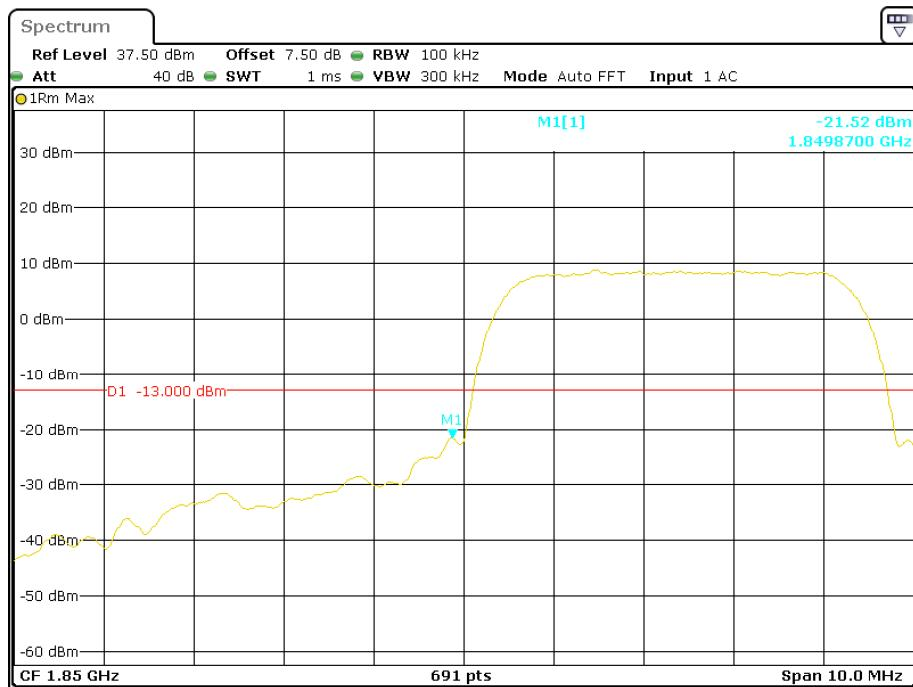
**PCS Band, Right Band Edge for HSDPA (16QAM) Mode**
