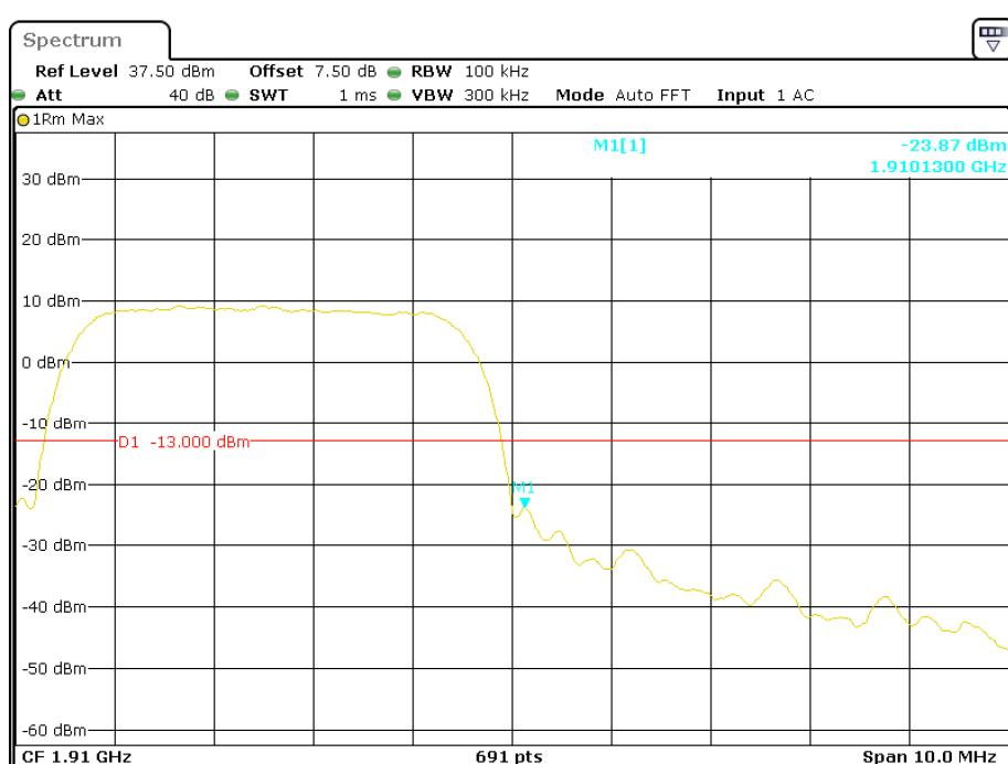
**PCS Band, Left Band Edge for HSUPA (BPSK) Mode**
