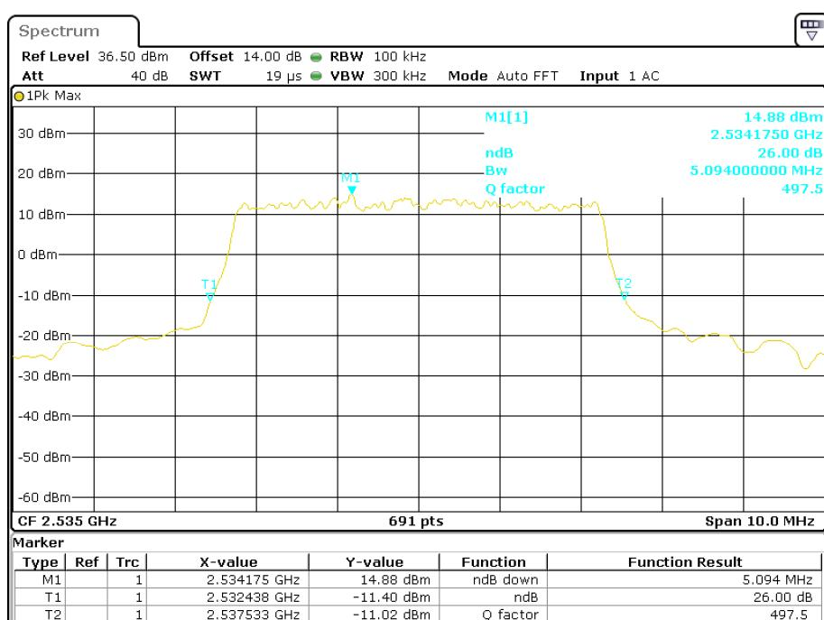
**QPSK (10.0 MHz) - 26 dB Bandwidth, Middle channel**
