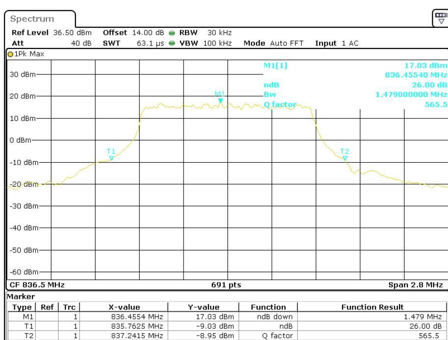
**QPSK (3.0 MHz) - 26 dB Bandwidth, Middle channel**
