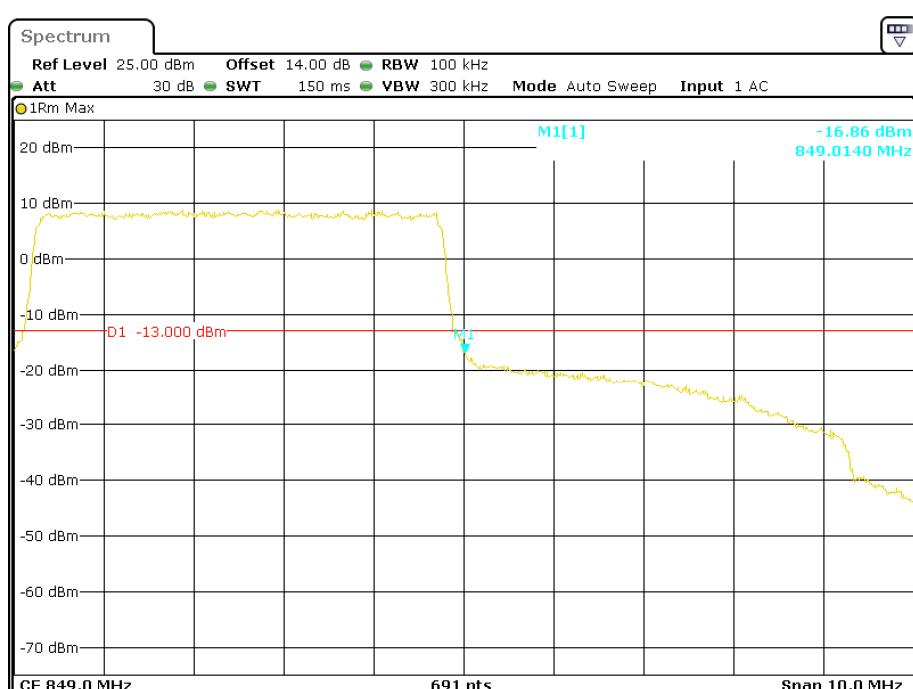
**QPSK (10.0 MHz, FULL RB) - Left Band Edge**
