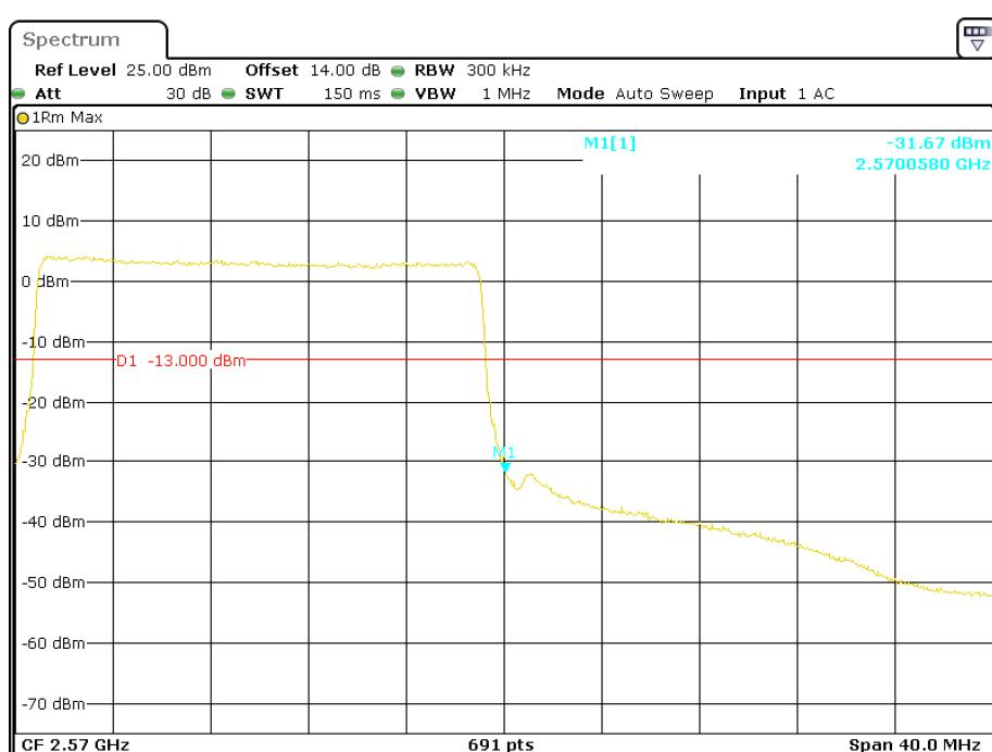
**16-QAM (20 MHz, FULL RB) - Left Band Edge**
