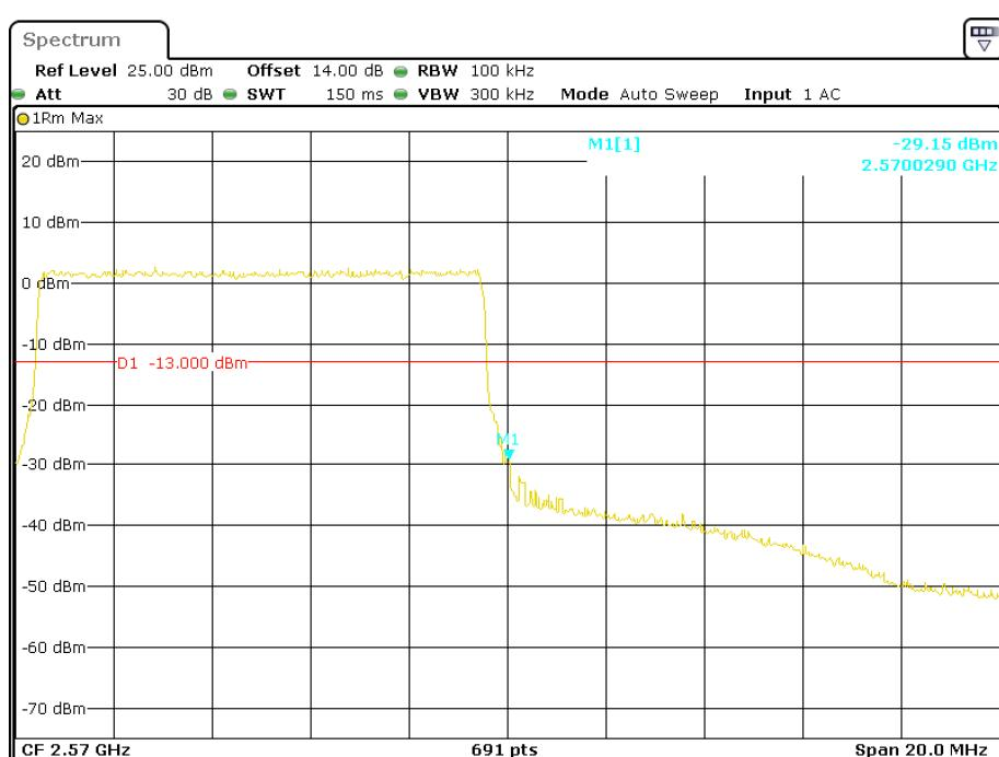
**16-QAM (10.0 MHz, FULL RB) - Left Band Edge**
