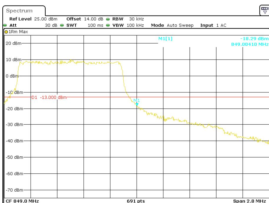
**QPSK (3.0 MHz, FULL RB) - Left Band Edge**
