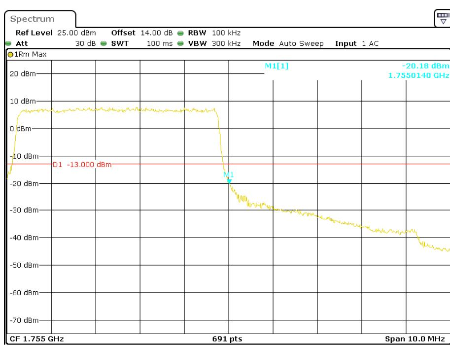
**16-QAM (5.0 MHz, FULL RB) - Left Band Edge**
