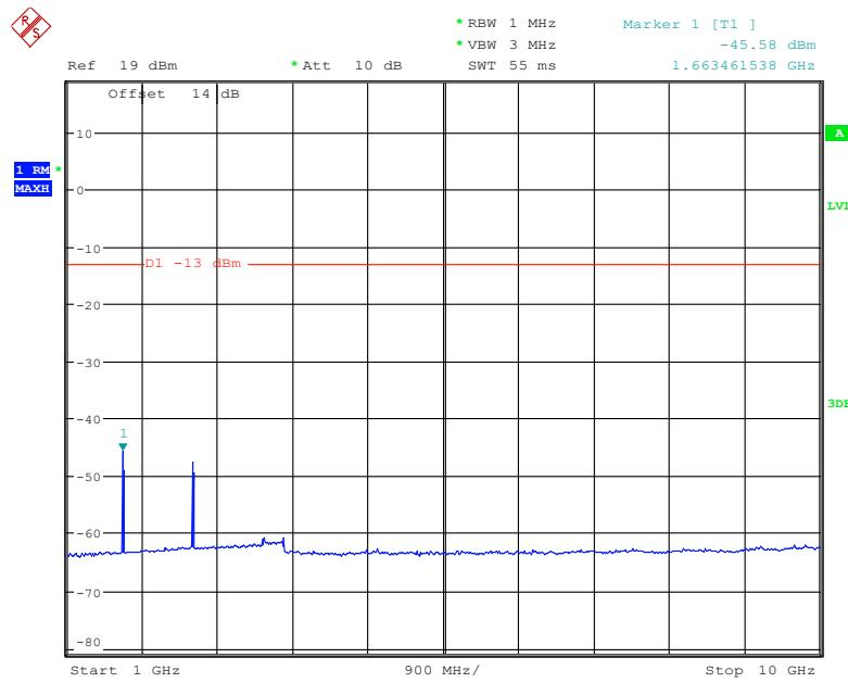
**LTE Band 7: (QPSK)****30 MHz - 1 GHz (5.0 MHz, Middle Channel)**
