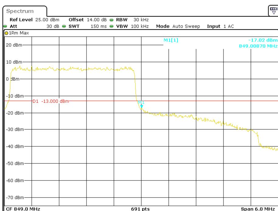
**16-QAM (3.0 MHz, FULL RB) - Left Band Edge**
