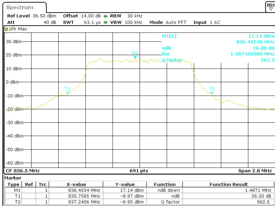
**16-QAM (1.4 MHz) - 26 dB Bandwidth, Middle channel**
