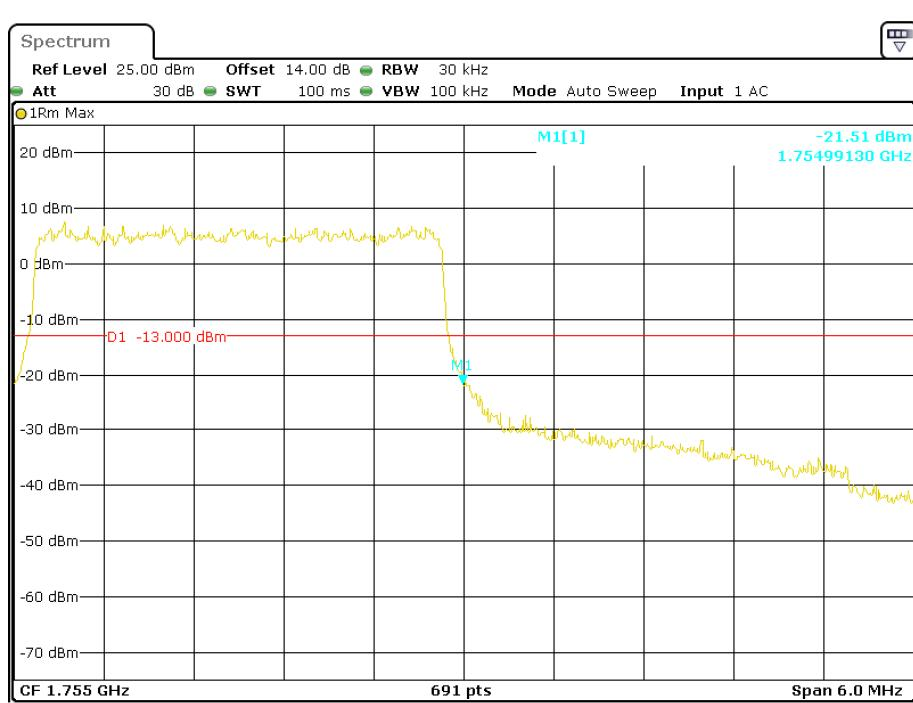
**QPSK (5.0 MHz, FULL RB) - Left Band Edge**
