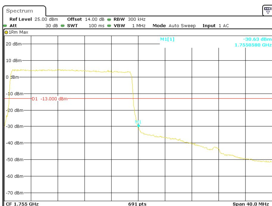
**16-QAM (20.0 MHz, FULL RB) - Left Band Edge**
