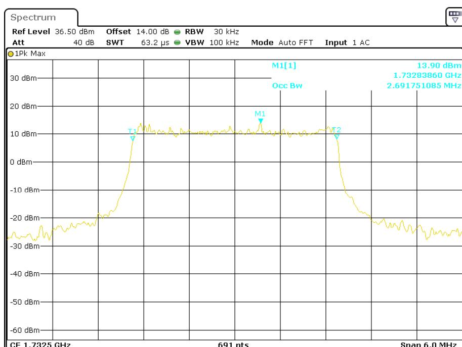
**QPSK (5.0 MHz) - 99% Occupied Bandwidth, Middle channel**
