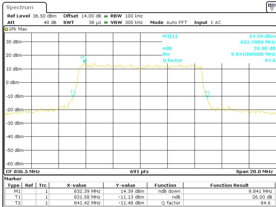
**16-QAM (10.0 MHz) - 26 dB Bandwidth, Middle channel**
