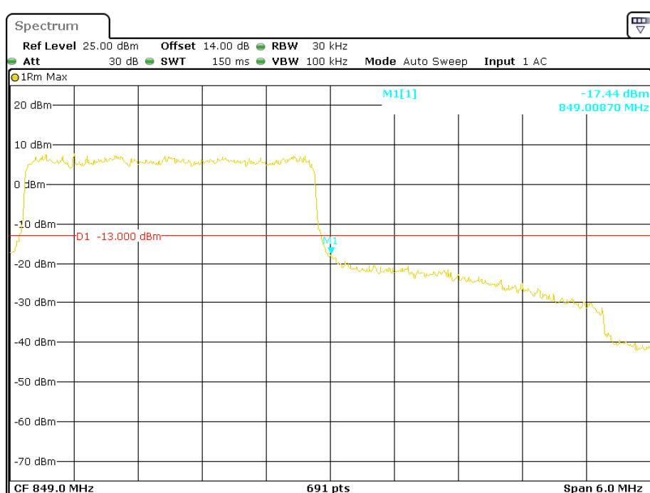
**QPSK (5.0 MHz, FULL RB) - Left Band Edge**
