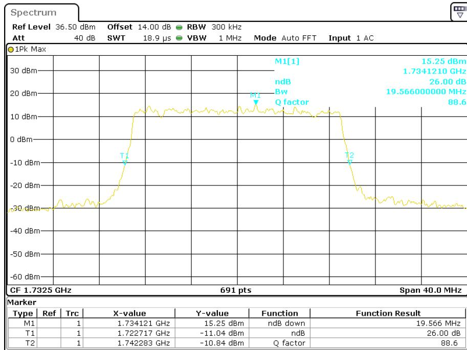
**16-QAM (20.0 MHz) - 26 dB Bandwidth, Middle channel**
