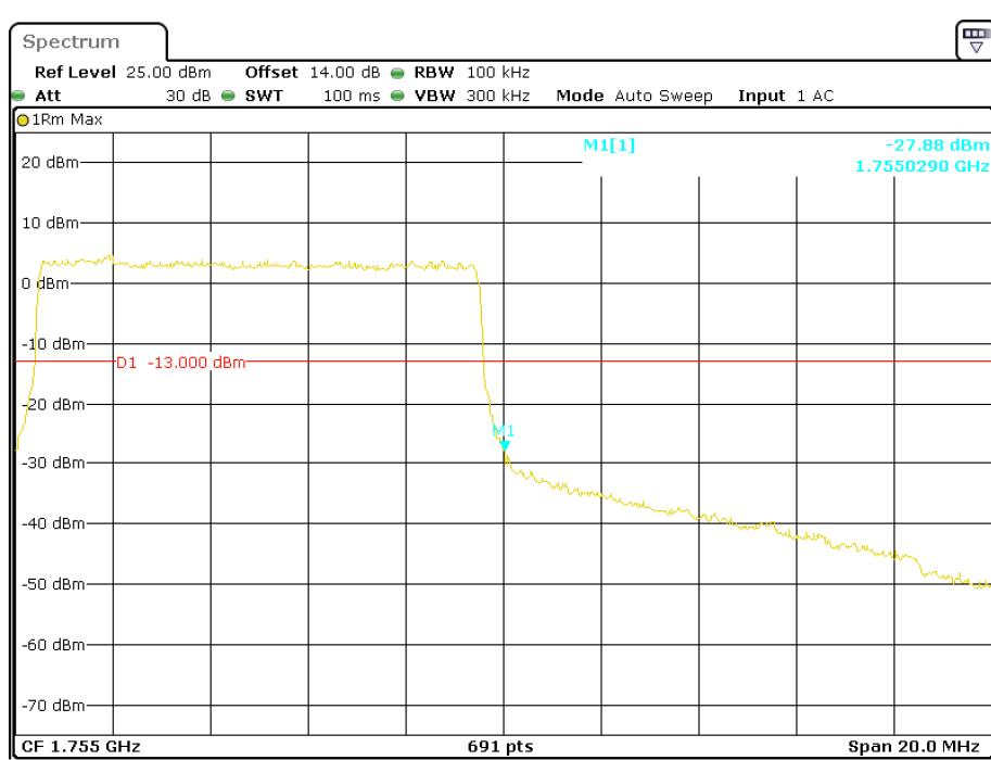
**16-QAM (10.0 MHz, FULL RB) - Left Band Edge**
