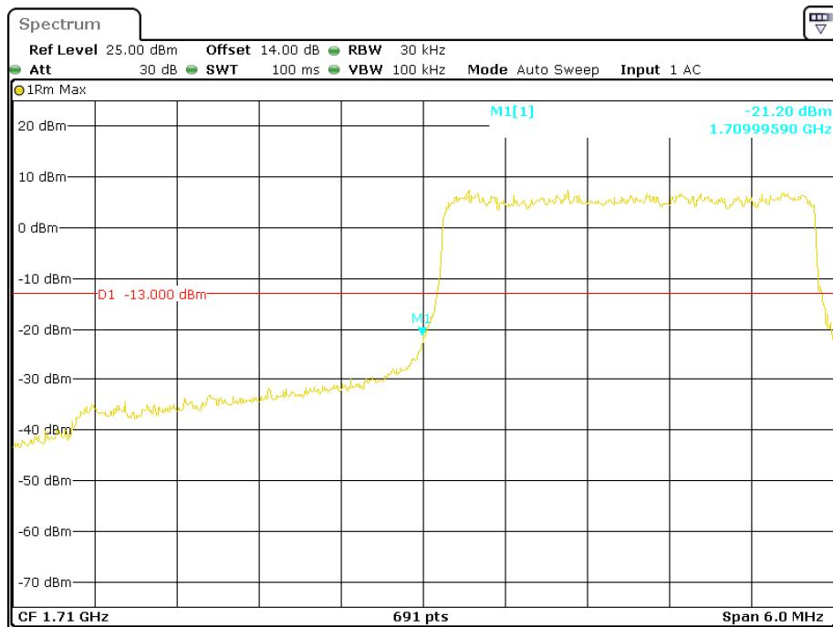
**16-QAM (3.0 MHz, FULL RB) - Right Band Edge**
