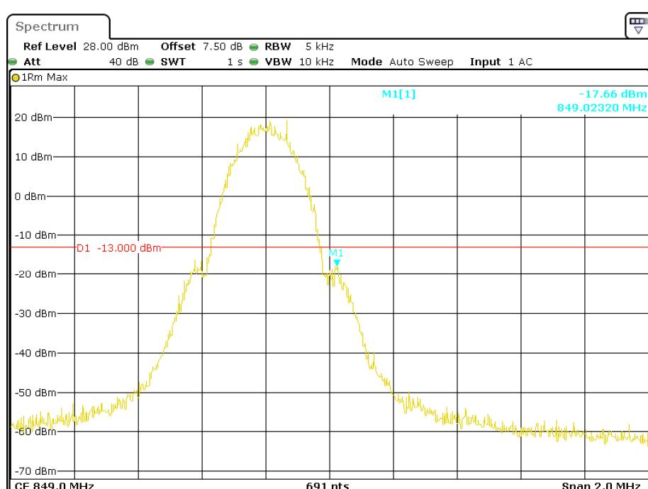
**Cellular Band, Left Band Edge for EDGE Mode**
