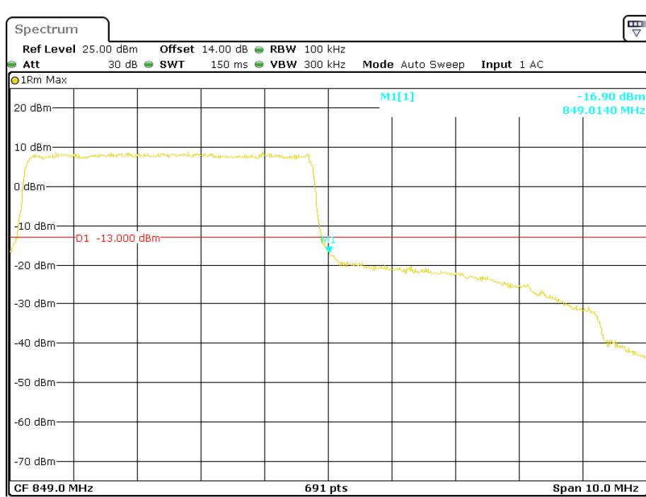
**16-QAM (5.0 MHz, FULL RB) - Left Band Edge**
