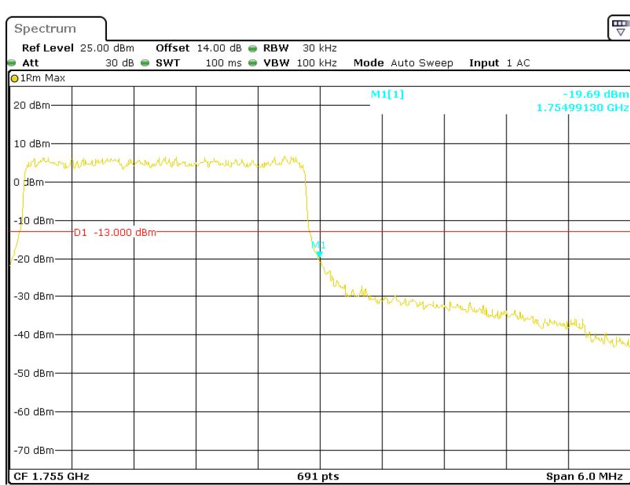
**16-QAM (3.0 MHz, FULL RB) - Left Band Edge**
