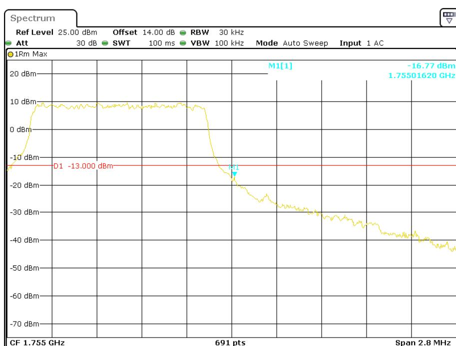
**QPSK (3.0 MHz, FULL RB) - Left Band Edge**
