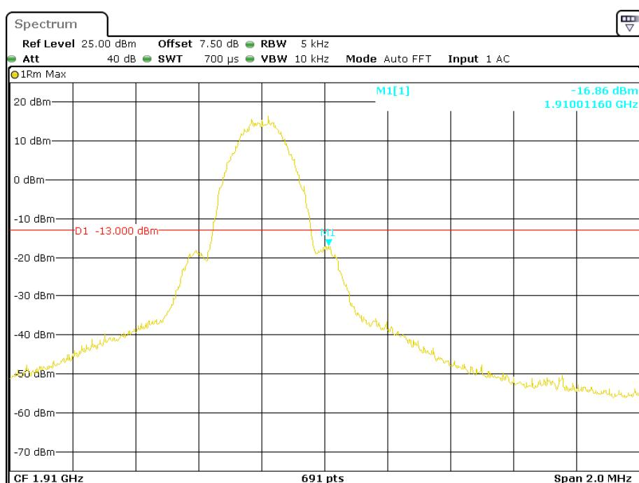
**PCS Band, Left Band Edge for WCDMA (BPSK) Mode**
