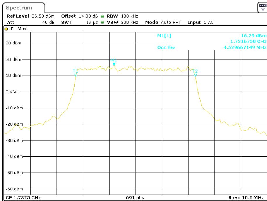
**16-QAM (5.0 MHz) - 99% Occupied Bandwidth, Middle channel**
