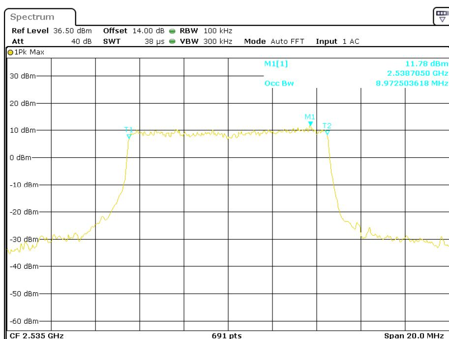
**QPSK (15.0 MHz) - 99% Occupied Bandwidth, Middle channel**
