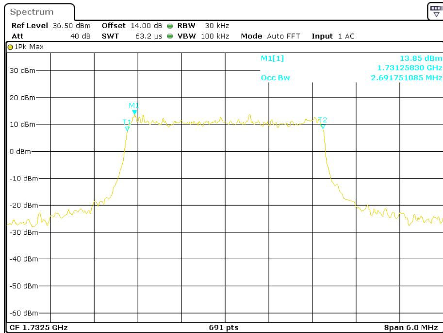
**16-QAM (3.0 MHz) - 99% Occupied Bandwidth, Middle channel**
