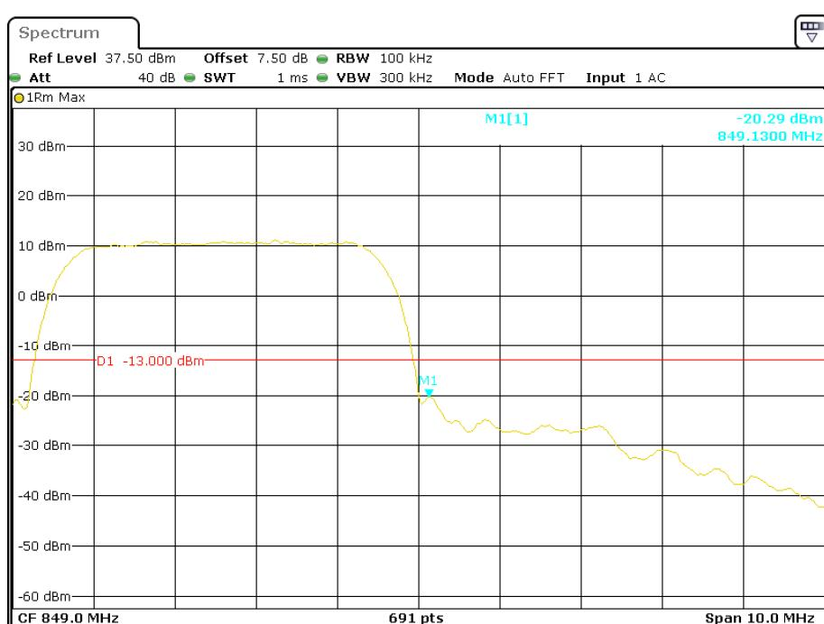
**Cellular Band, Left Band Edge for HSUPA (BPSK) Mode**
