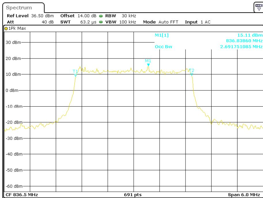
**16-QAM (3.0 MHz) - 99% Occupied Bandwidth, Middle channel**
