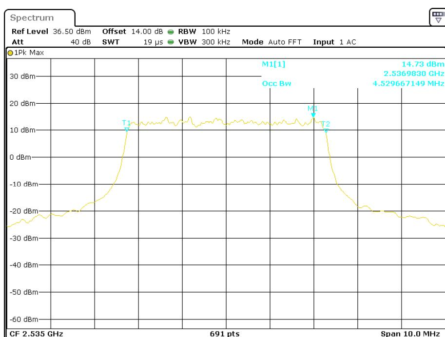
**QPSK (10.0 MHz) - 99% Occupied Bandwidth, Middle channel**
