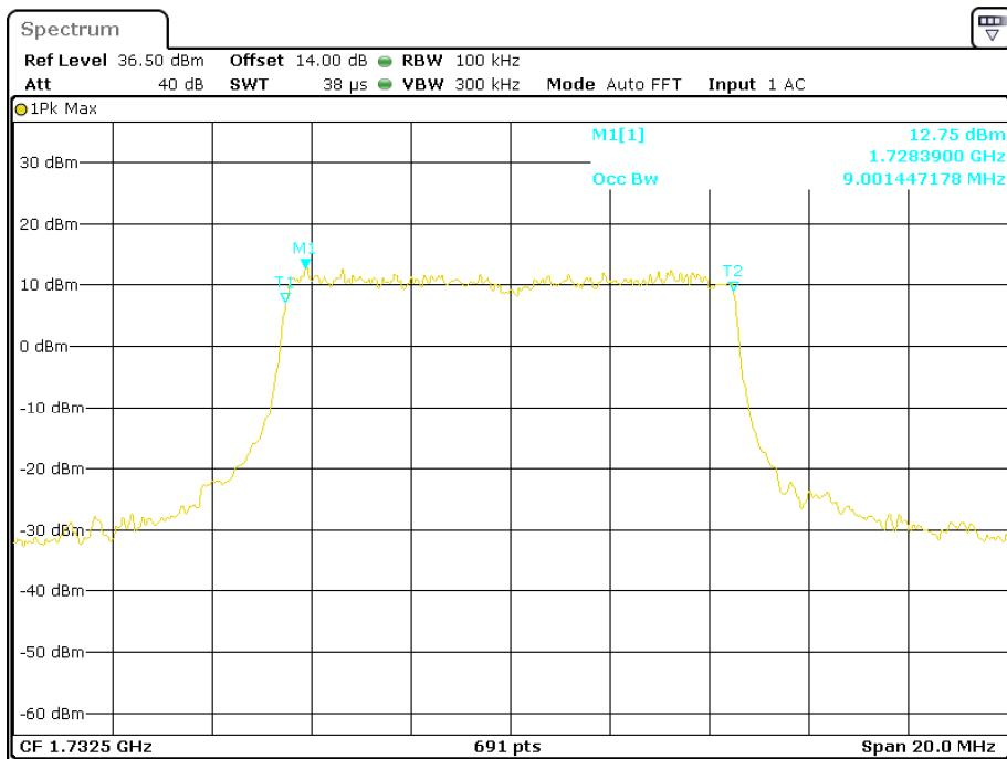
**16-QAM (10.0 MHz) - 99% Occupied Bandwidth, Middle channel**
