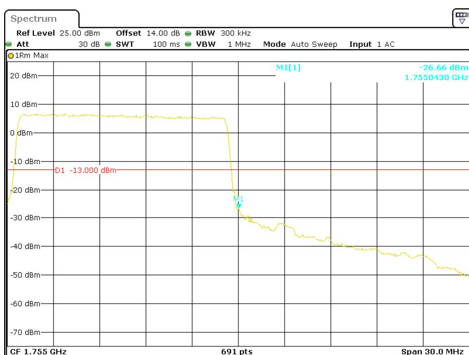
**16-QAM (15.0 MHz, FULL RB) - Left Band Edge**
