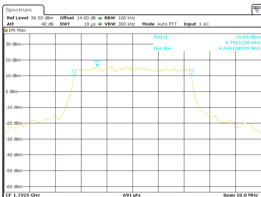
**QPSK (10.0 MHz) - 99% Occupied Bandwidth, Middle channel**
