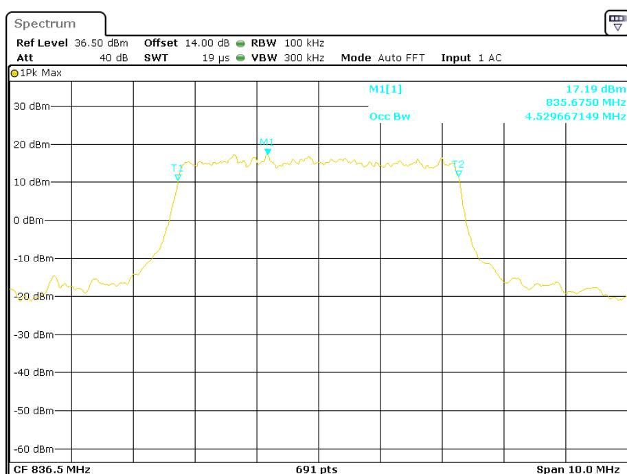
**QPSK (10.0 MHz) - 99% Occupied Bandwidth, Middle channel**
