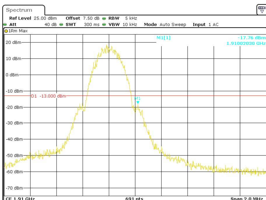
**PCS Band, Left Band Edge for EDGE Mode**
