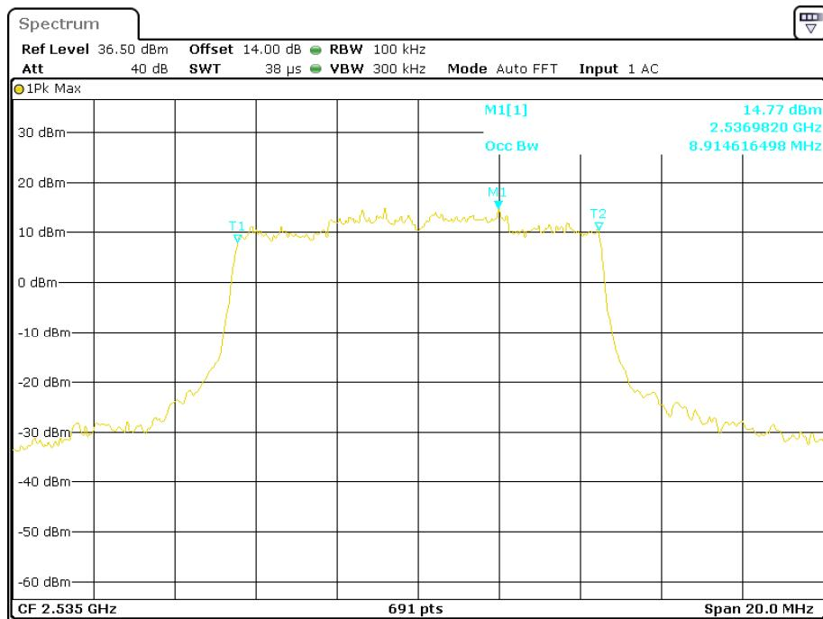
**16-QAM (10.0 MHz) - 99% Occupied Bandwidth, Middle channel**
