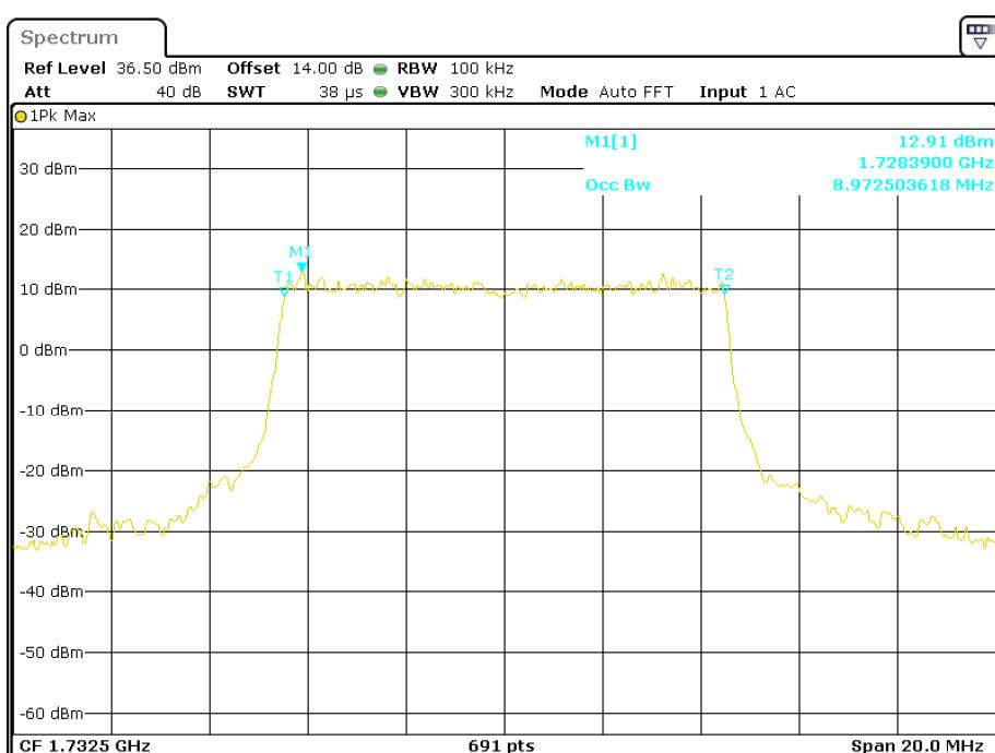
**QPSK (15.0 MHz) - 99% Occupied Bandwidth, Middle channel**
