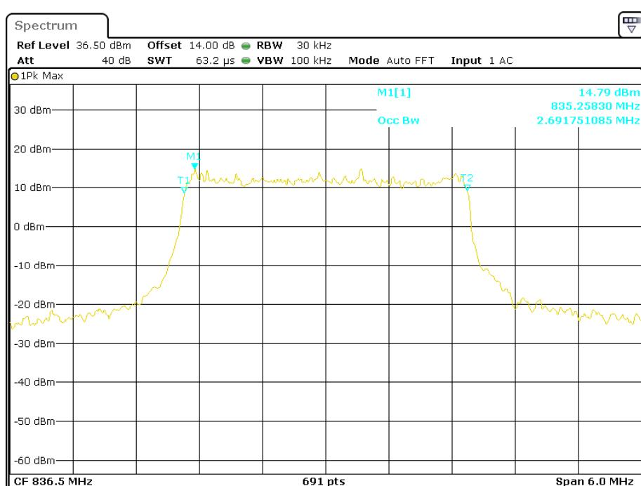
**QPSK (5.0 MHz) - 99% Occupied Bandwidth, Middle channel**
