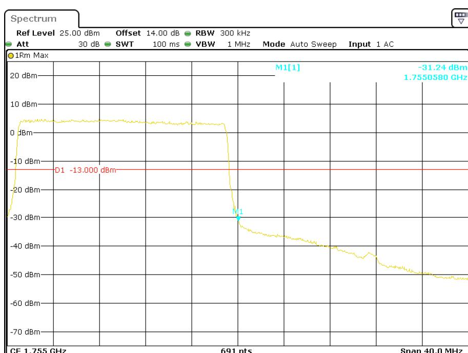
**Band 5:****QPSK (1.4MHz, FULL RB) - Left Band Edge**
