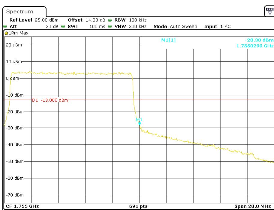
**QPSK (15.0 MHz, FULL RB) - Left Band Edge**
