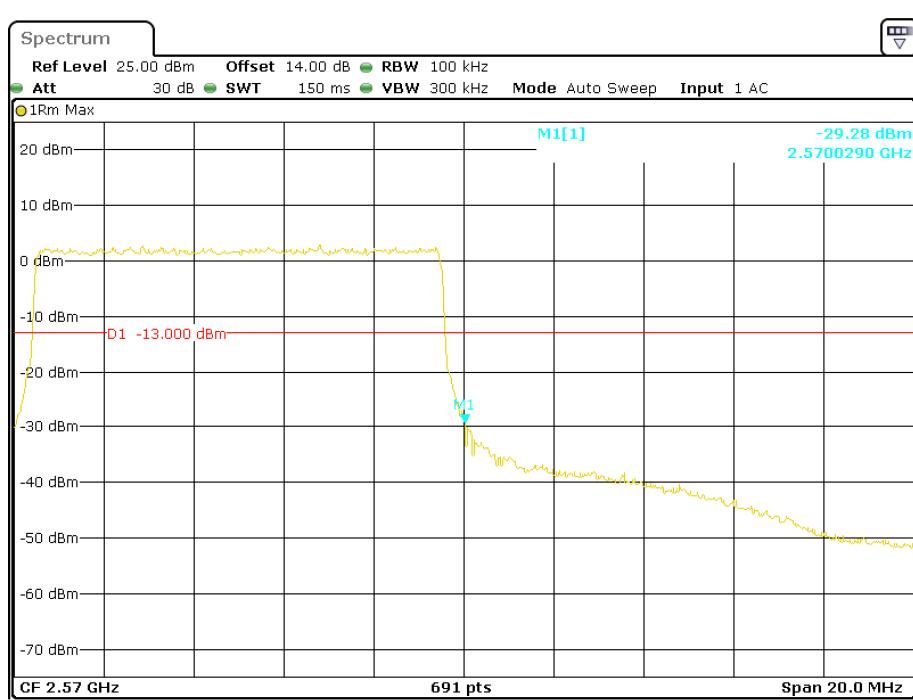
**QPSK (15 MHz, FULL RB) - Left Band Edge**
