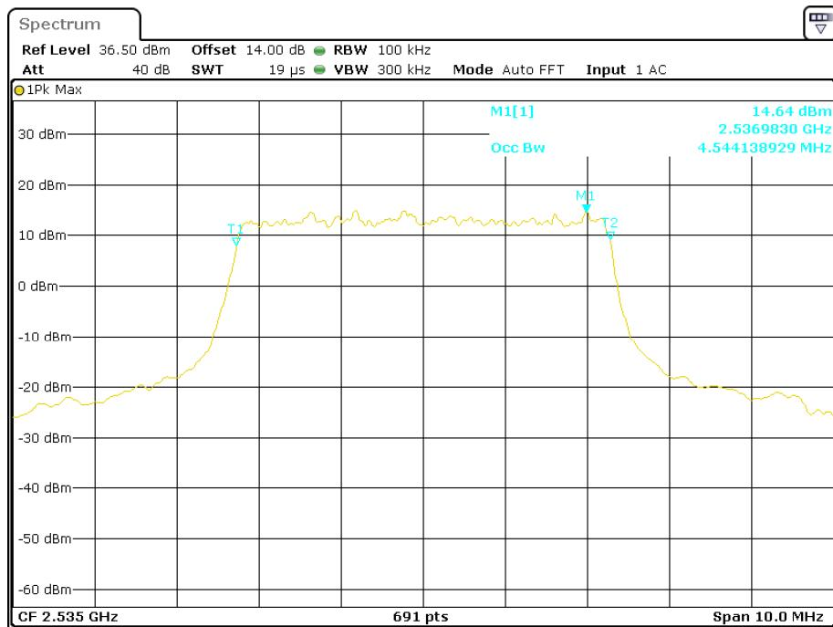
**16-QAM (5.0 MHz) - 99% Occupied Bandwidth, Middle channel**
