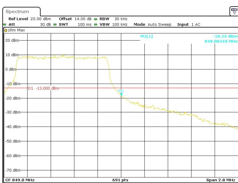
**16-QAM (1.4 MHz, FULL RB) - Left Band Edge**
