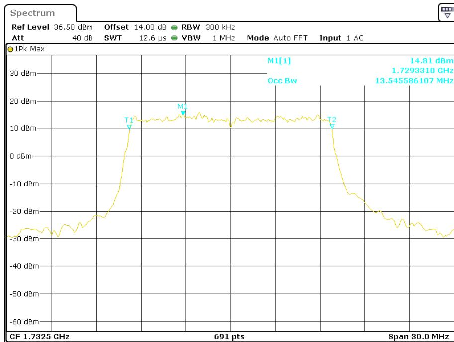
**16-QAM (15.0 MHz) - 99% Occupied Bandwidth, Middle channel**
