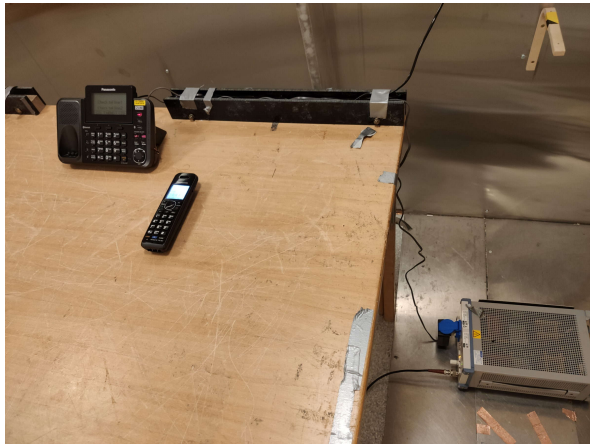
Power-Line Conducted Emissions
