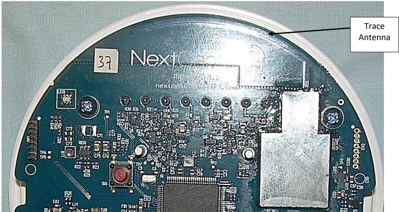
**Photograph 4 – 900MHz Trace Antenna**
