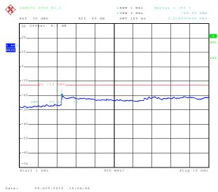
8.2.1.5 Out of Band Emissions at Antenna Terminals GMSK, PCS Middle channel, 1880.0 MHz, 2 Hz to 1 GHz
