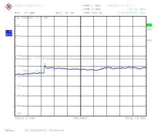
8.2.1.3 Out of Band Emissions at Antenna Terminals 8-PSK, Cell Mid Channel, 836.6 MHz, 2 Hz to 1 GHz
