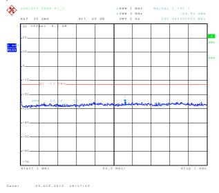
8.2.1.9 Out of Band Emissions at Antenna Terminals 8-PSK, PCS Middle channel, 1880.0 MHz, 1GHz to 10 GHz
