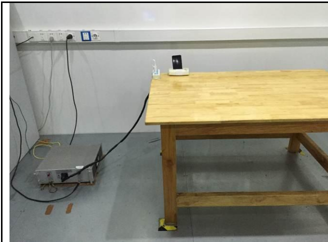
Conducted Emissions Test Setup Front View
