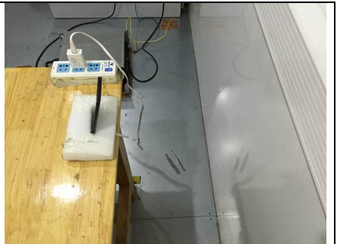
Conducted Emissions Test Setup Side View
