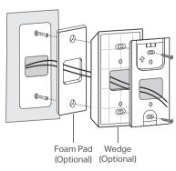
3. Connect the wires to the two terminals at the back of the doorbell, then tighten the terminal screws.
