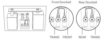
4. Tighten the screws and replace the chime cover.
