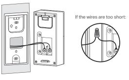
4. Mount the doorbell to the bracket and turn on the circuit breaker.
