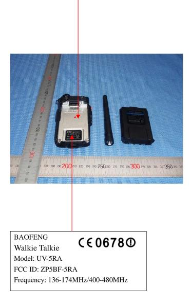
Note: The label shown shall be permanently affixed at a conspicuous location on the device and be readily visible to the user at the time purchase
