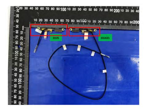
Include a dimensioned photo and dimensioned drawing of Main antenna here.
