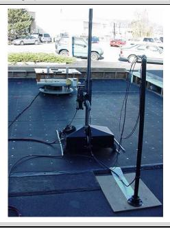
Photograph J.7-4 - Mobile - 3 m Horn Setup
