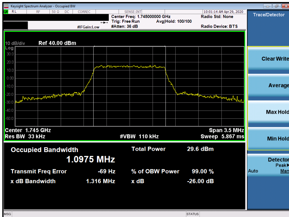
Plot 7-18. Occupied Bandwidth Plot (LTE Band 66/4 - 1.4MHz 64-QAM - Full RB Configuration)
