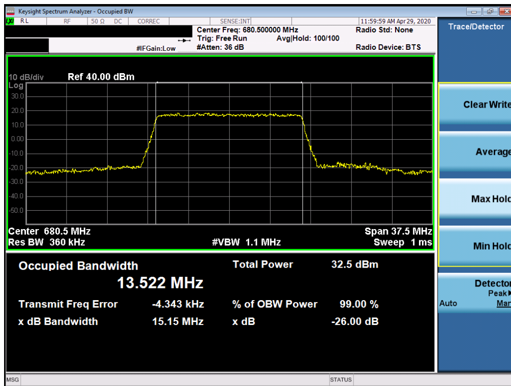
Plot 7-40. Occupied Bandwidth Plot (LTE Band 71 - 15MHz QPSK - Full RB Configuration)
