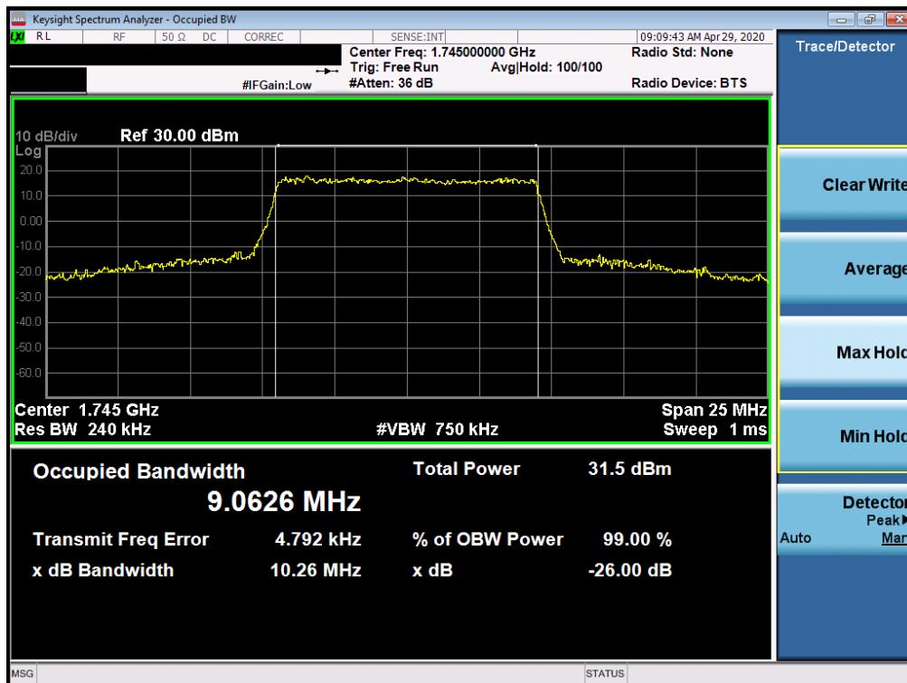
Plot 7-8. Occupied Bandwidth Plot (LTE Band 66/4 - 10MHz 16-QAM - Full RB Configuration)
