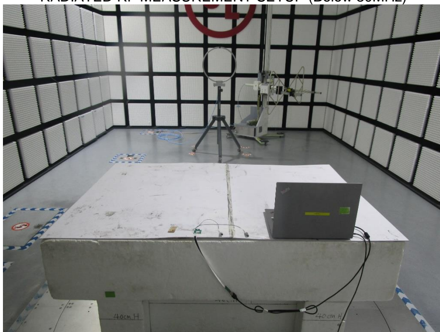
RADIATED RF MEASUREMENT SETUP (Below 30MHz)
