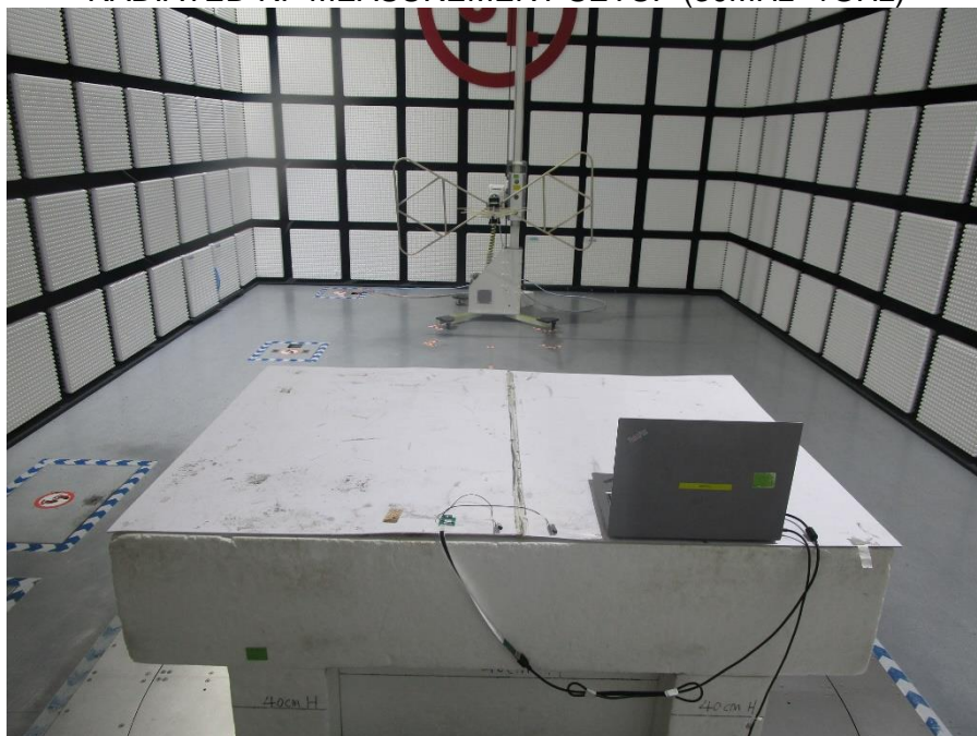
RADIATED RF MEASUREMENT SETUP (Below 30MHz)
