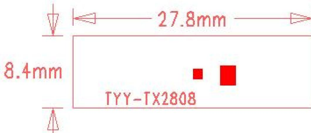
Figure 2 WIFI main antenna TYY-TX2808 (cable length 110mm, with 1st generation terminal)
