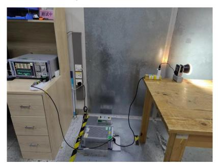
Radiated Emissions From 30MHz-1000MHz
