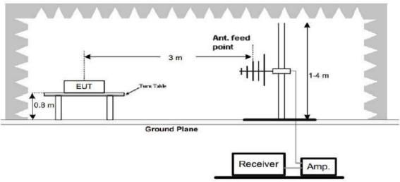
3. Radiated Emission Test-Up Frequency Above 1GHz
