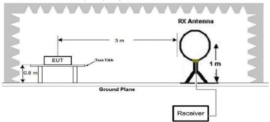
2. Radiated Emission Test-Up Frequency 30MHz~1GHz
