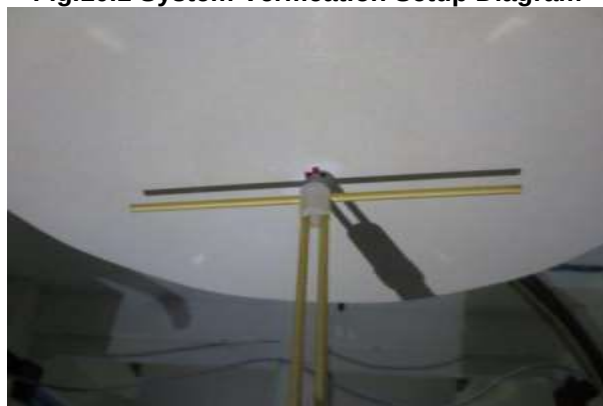
Fig.10.2 Photo of Dipole setup
