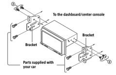
When mounting this unit to the preinstalled brackets of your car, use the mounting screws (2) in the appropriate screw holes based on your car: T for TOYOTA and N for NISSAN.
