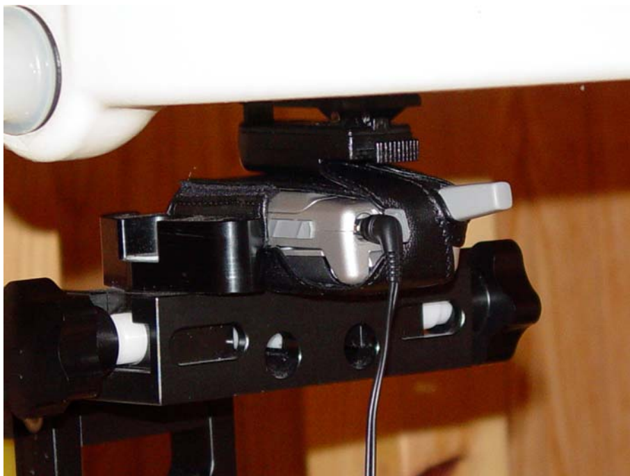
Figure 10.5 body SAR setup (with leather case)
