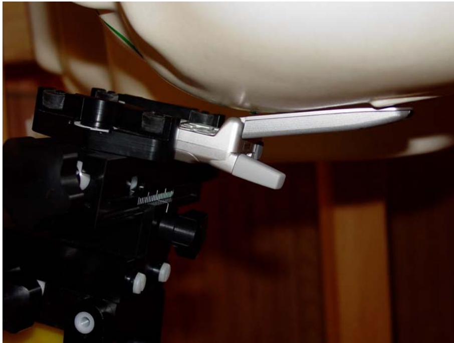
Figure 10.2 phone against the head (left cheek position)
