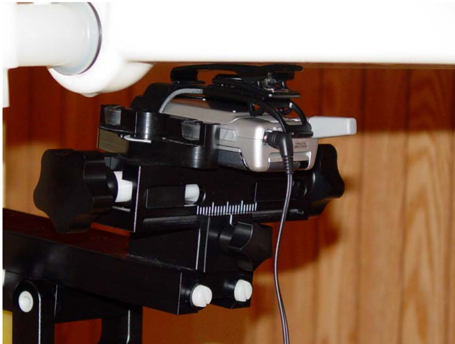
Figure 10.4 body SAR setup (with holster)
