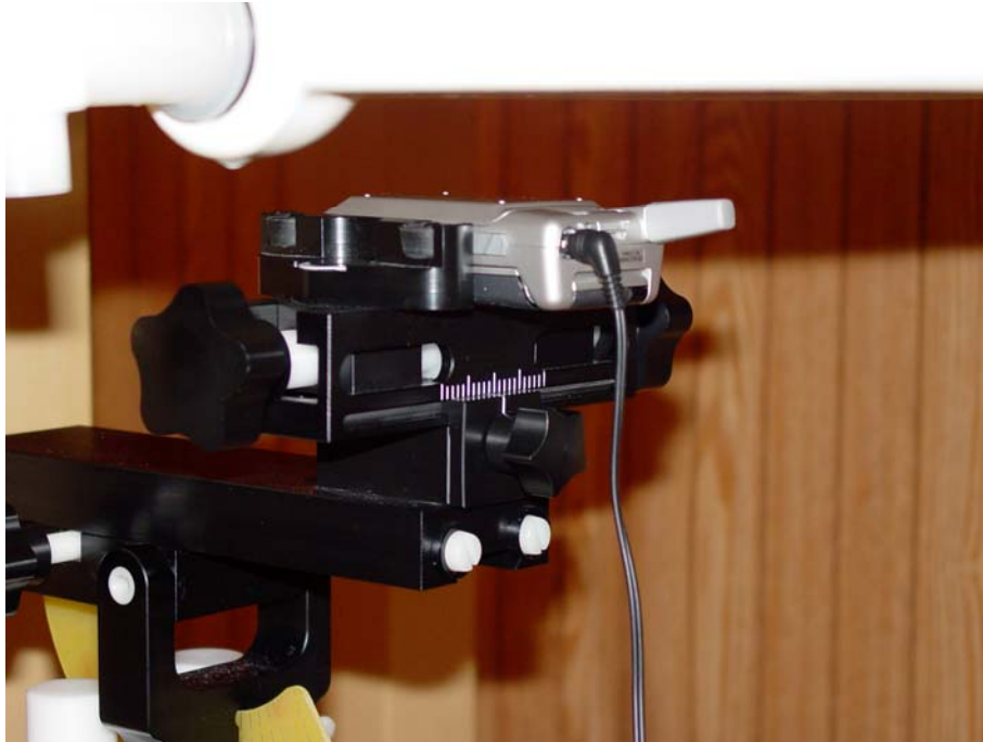
Figure 10.6 body SAR setup (with 25mm air separation)
